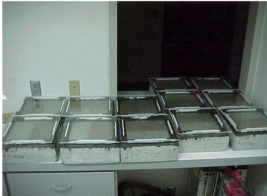
Figure 4.5 Houston Samples Ponded for 180 Days
