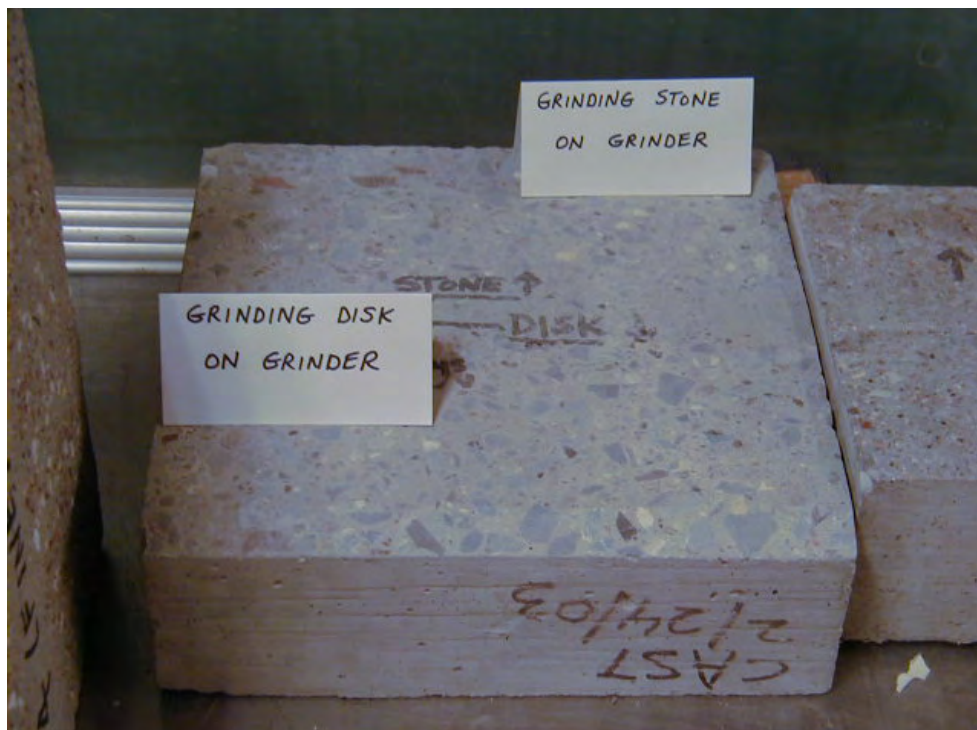
Figure 4.2 Sample Abraded Using Grinding Technique
