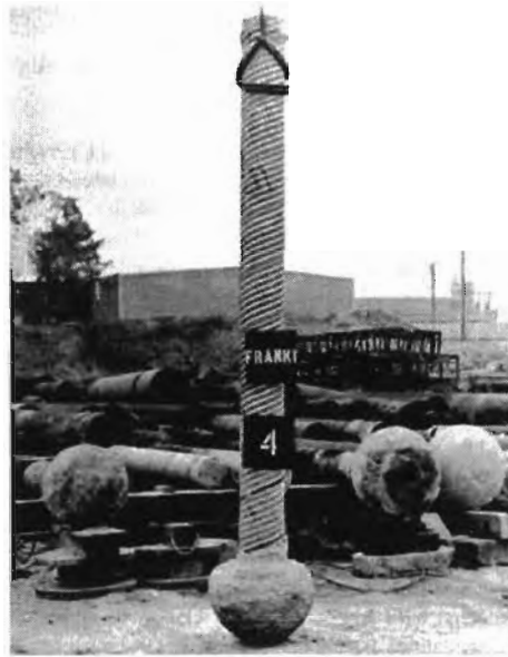
Figure 2.7 Extracted Cased Shaft PIF with a 24” Base Diameter (Source: “Foundation Design Principles and Practice”, Donald P. Coduto, Prentice Hall, Inc., Copyright 2001, Figure 11.49, page 428)
