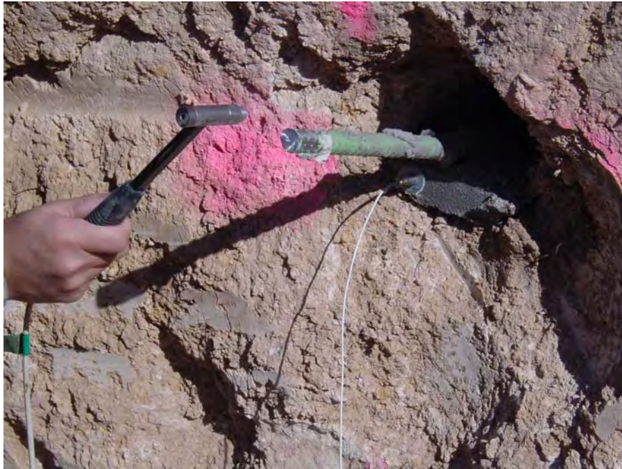
Figure 5.6 Sonic Echo and Impact Echo Test Configuration: Accelerometer Mounted on the Grout, Impact on the Steel Tendon with the Alumina Tip
