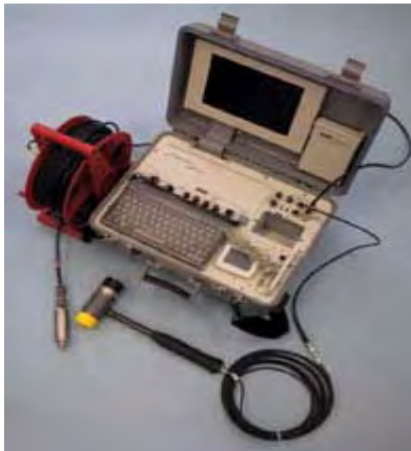
Figure 3.18 Test Equipment for Parallel Seismic Method
