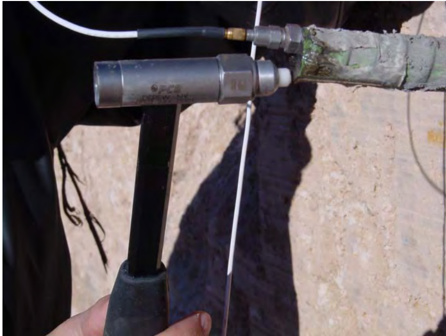
Figure 5.8 Sonic Echo and Impact Echo Test Configuration: Accelerometer Mounted on the Steel Tendon, Impact on the Steel Tendon with the Plastic Tip
