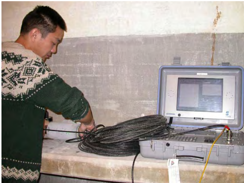
Figure 5.15 Ultrasonic Pulse Velocity Testing Configuration
