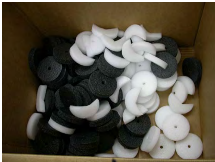
Figure 4.7 Polyethylene Foam Disks Used in Defect Simulation
