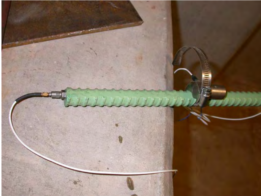
Figure 5.29 Laboratory Sonic Echo Tests on Standalone Steel Tendon
