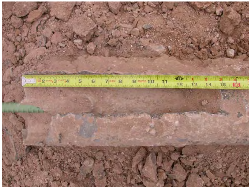
Figure 5.52 Bird’s Mouth Defect Observed in Test Nail No.11
