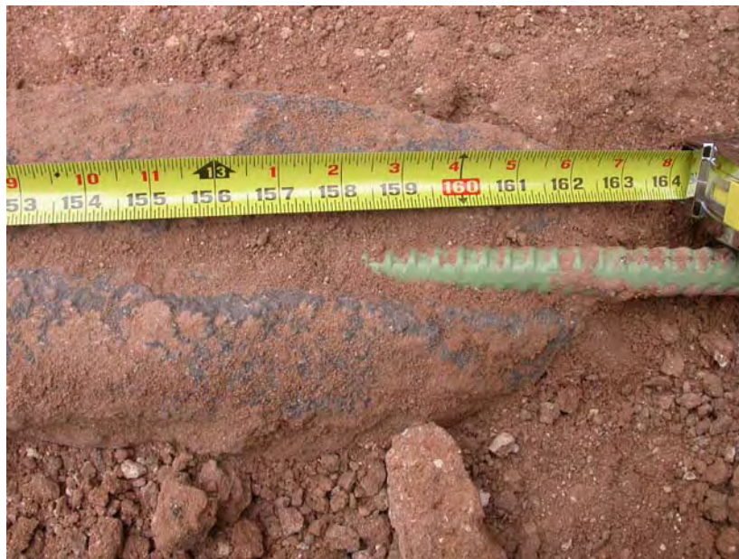
Figure 5.39 Nail No. 7 – Grout Ends at 13.6ft
