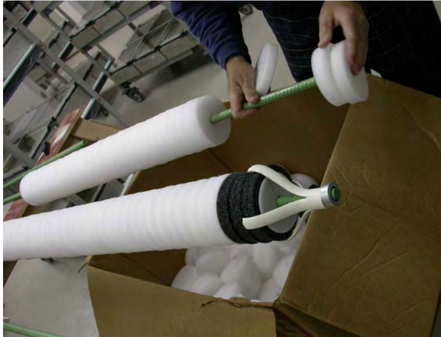
Figure 4.8 Mounting Foam Disks on Steel Tendons
