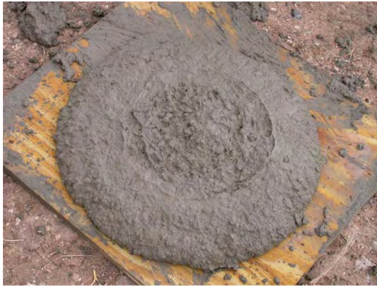
Figure 6.7 Puddle Remaining After Slump Test of 11-inch Slump Sand-Cement Grout
