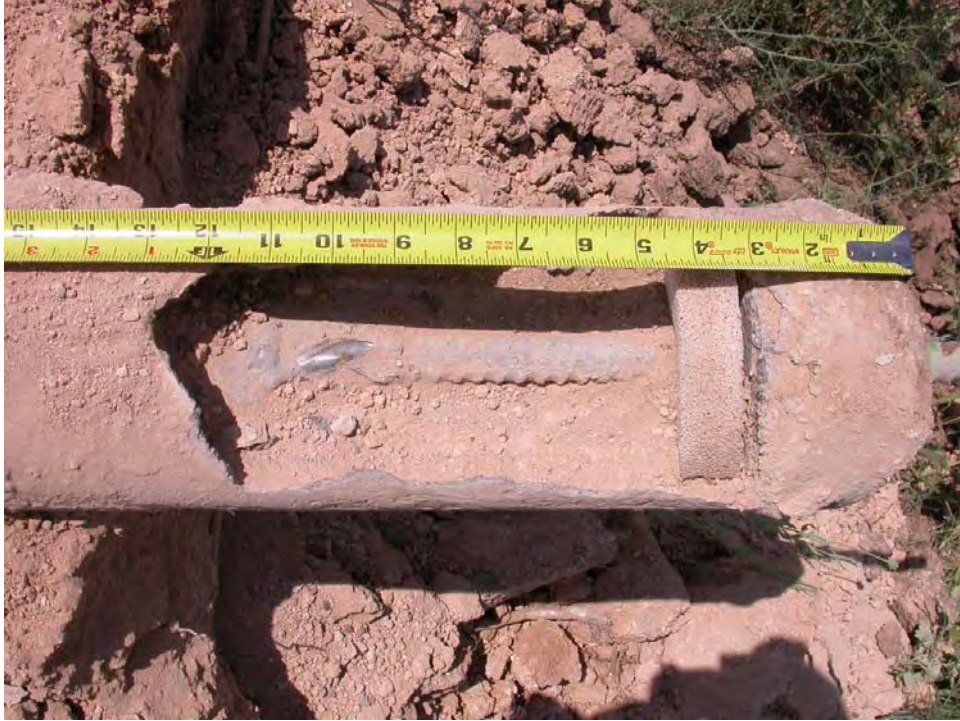
Figure 5.57 Bird's Mouth Observed in Nail No.23
