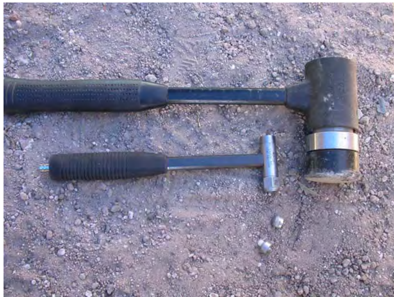
Figure 5.2 Modulated PCB Hammers with Alumina and Plastic Tips
