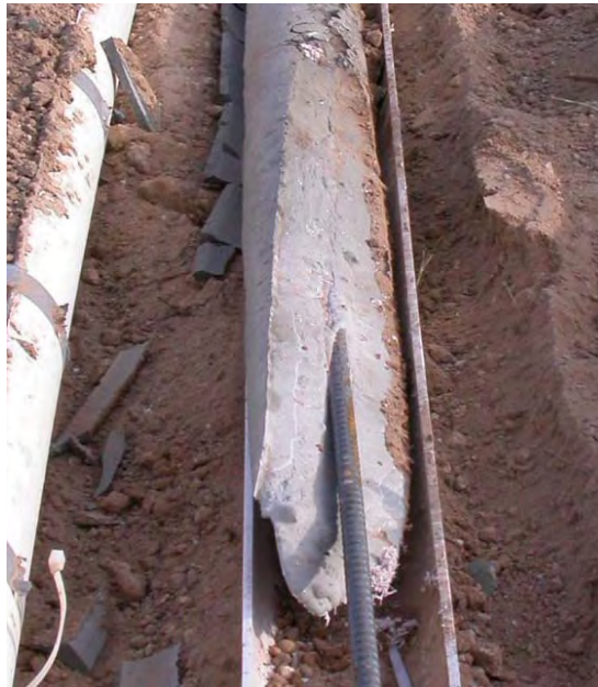
Figure 6.10 Reposed Tail on the Downhole End of the Minimally Tremied Neat Cement Grout Tube
