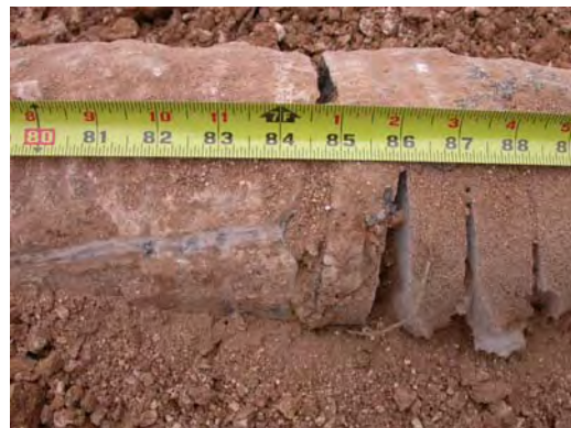
Grout ends at 7'
