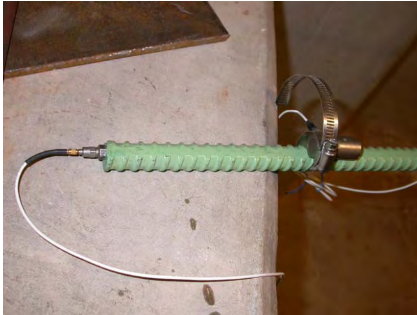
Figure 5.3 An Accelerometer being Used for Receiving Feedback Signal
