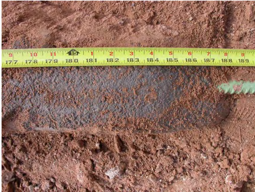
Figure 5.43 Nail No.16 Grout Ends at 15ft 8in
