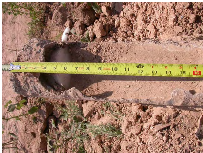
Figure 5.55 Bird's mouth Observed in Nail No.17
