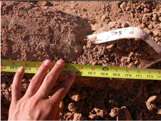
Grout lost half cross section at 14'
