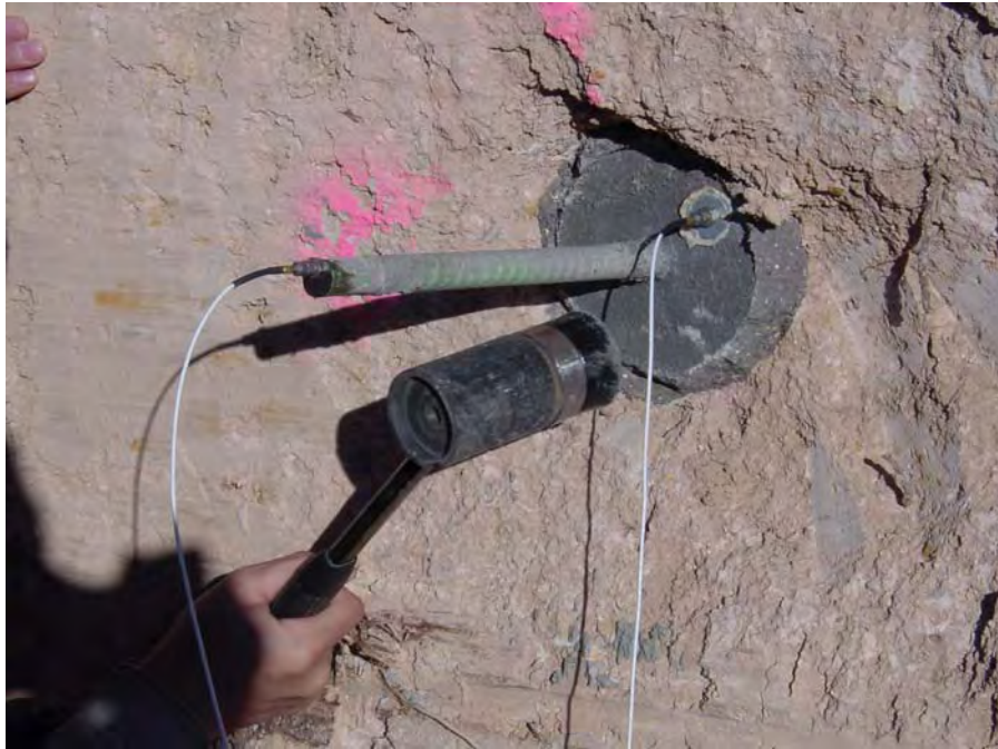
Figure 5.10 Impulse Response Configuration: Accelerometers Mounted on the Grout and the Steel Tendon, Impact on the Grout
