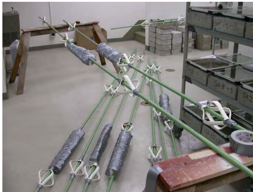
Figure 4.9 Soil Nail Tendons with Foam Disks Mounted to Simulate Voids at the Middle of the Nail
