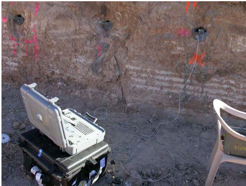
Figure 5.5 Freedom Data PC Connected to Sensors and Impactor
