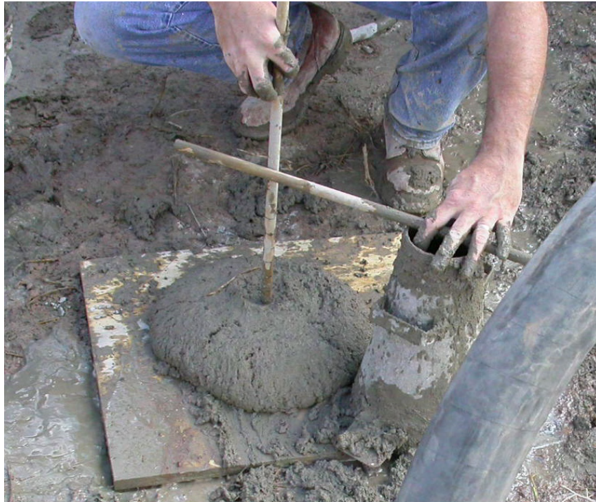
Figure 6.6 ASTM Slump Test of Sand-Cement Grout in Progress
