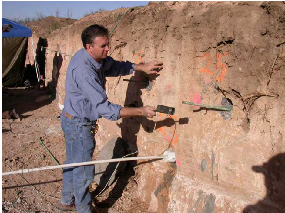
Figure 5.18 Parallel Seismic Test Configuration
