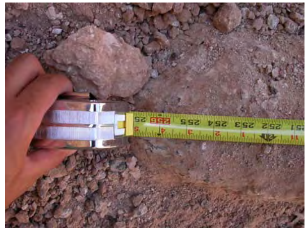
Figure 5.32 Grouted Length of Nail No.26 = 21 ft 5in
