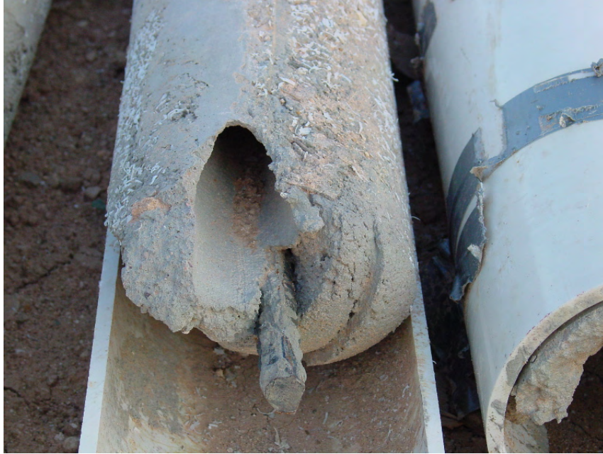
Figure 6.13 Sand Grout Column With A Defect Caused By Withdrawal Of The Tremie From The Surface Of The Grout As It Was Being Pumped
