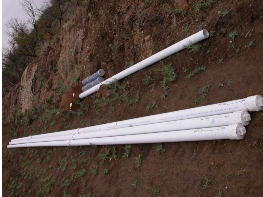
Figure 4.24 PVC Pipes Used as Access Tubes for NDT Instrumentation (Parallel & Cross-Hole Seismic Tests)
