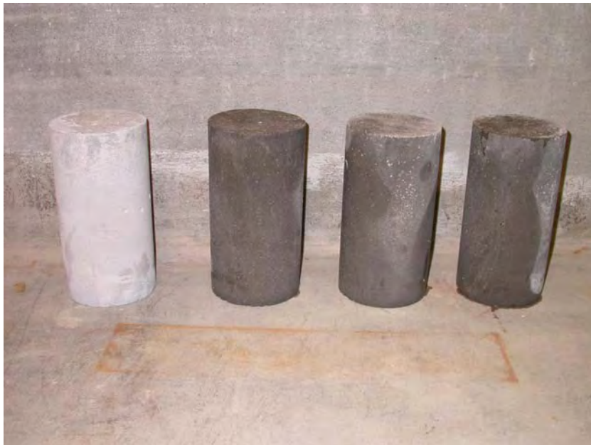
Figure 5.13 Grout Cylinder Used for Wave Velocity Calculation
