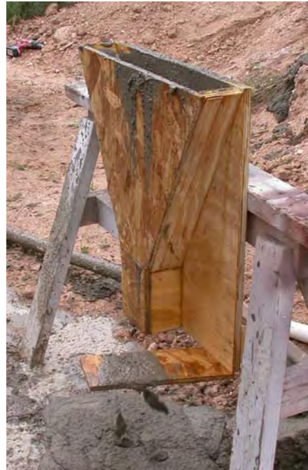
Figure 6.9 V-funnel Apparatus; Dimensions (left) and Test Apparatus in Use (right)
