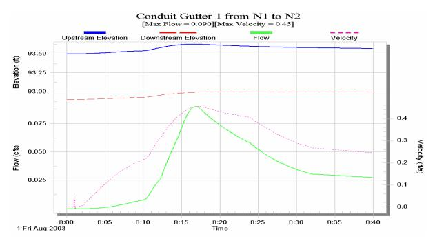
Figure D.33. Time series output from SWMM for conduit Gutter1.
