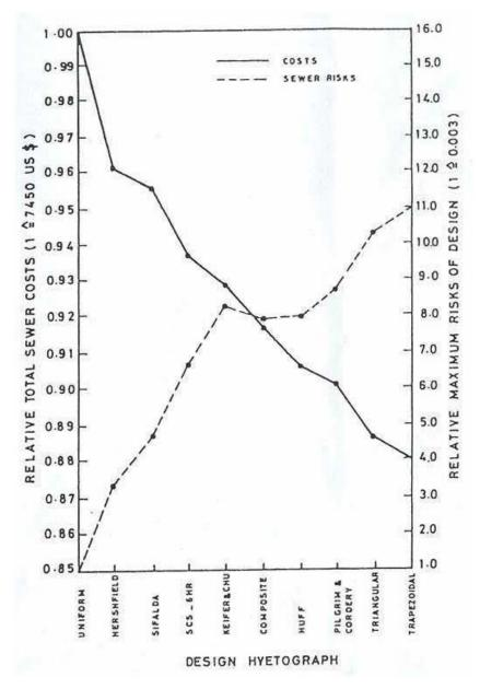
Figure 2.10 Effect of time distribution of rainfall on least-cost sewer system design (Nouh, 1987)
