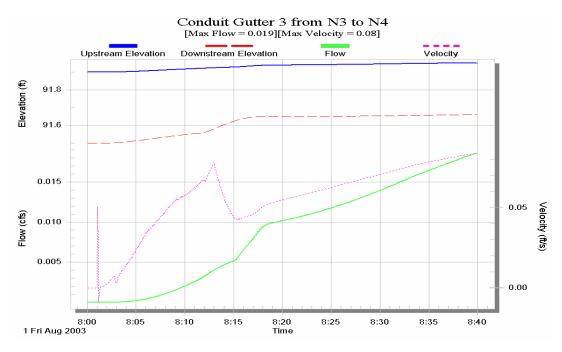
Figure D.37. Time series output from SWMM for conduit Gutter 3.
