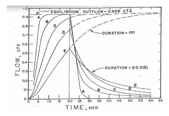
Figure D.6b. Sub-catchment hydrographs for different shapes of Figure D.6a (Huber, 1988).
