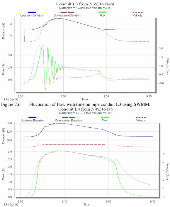
Figure 7.7 SWMM output of time distributed flow in pipe conduit L4.
