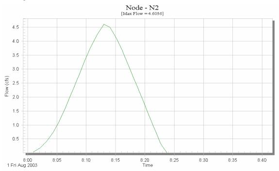
Figure D.16. SWMM output for Node-N2 solved in Runoff layer only ( $T_c = 10$  minutes).
