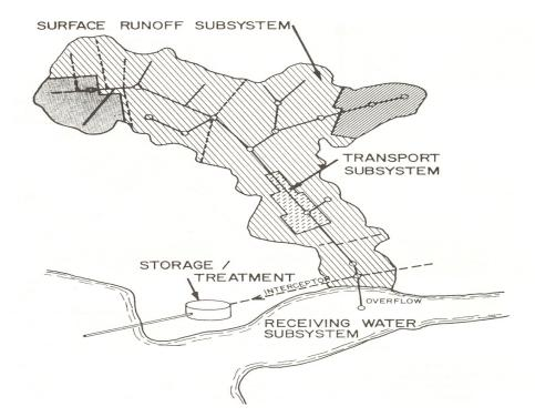
Figure 1.1 The urban drainage system (from Proctor and Redfern, 1976).
