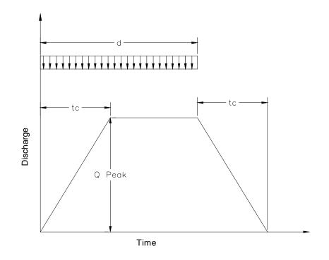
Figure 2.2(a) Hydrograph when duration of rainfall is greater than  $t_c$ .
