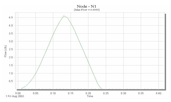
Figure D.12. Hydrograph output of SWMM for Node N1.
