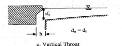
Figure 2.6. Curb opening inlets with different throats (Mays, 2001).
