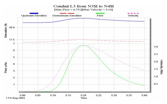
Figure D.36. Time series output from SWMM for conduit L-3.
