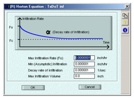
Figure D.3. Input parameters for Horton Equation in SWMM.
