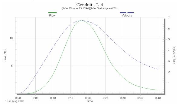
Figure D.15. Time series plot of flows and velocity by SWMM for conduit L4.
