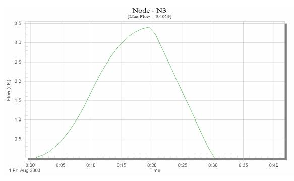
Figure D.17. SWMM output for Node-N3 solved in Runoff layer only.
