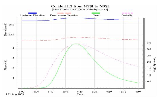
Figure D.34. Time series output from SWMM for conduit L-2.
