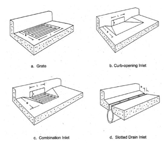
Figure 2.4. Types of storm drain inlets (Brown et al., 2001).
