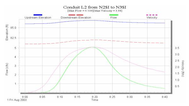
Figure D.24 Time series output of flow, velocity and elevation for conduit L2 resulted from Extran layer of SWMM for a maximum interception capacity of 3.0 cfs for inlet.
