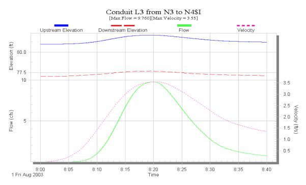
Figure D.22 Time series output of flow, velocity and elevation for conduit L-3 resulted from Extran layer of SWMM.
