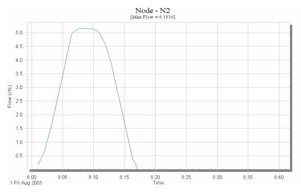
Figure D.19. SWMM output for Node-N2 solved in Runoff layer only ( $T_c = 5$  minutes).
