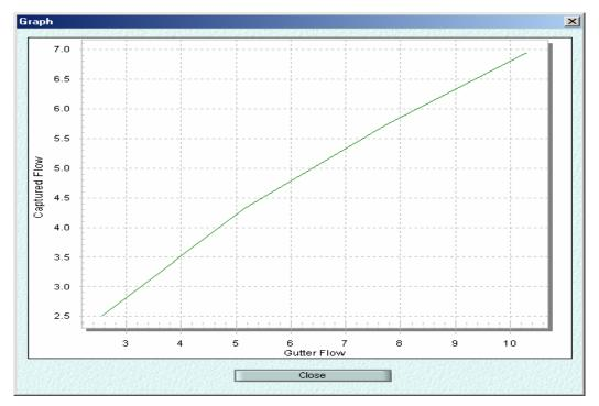
FigureD.10b. Graphical view of rating curve in Figure D.10a.
