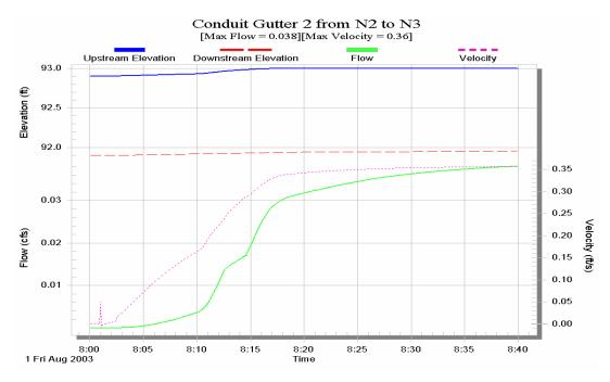
Figure D.35. Time series output from SWMM for conduit Gutter 2.
