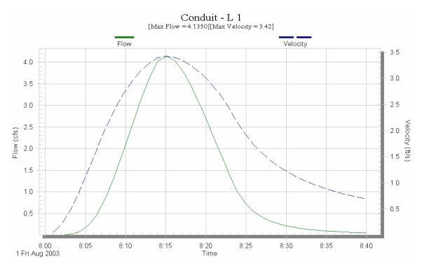
Figure D.13. Time series plot of flows and velocity by SWMM for conduit L1.
