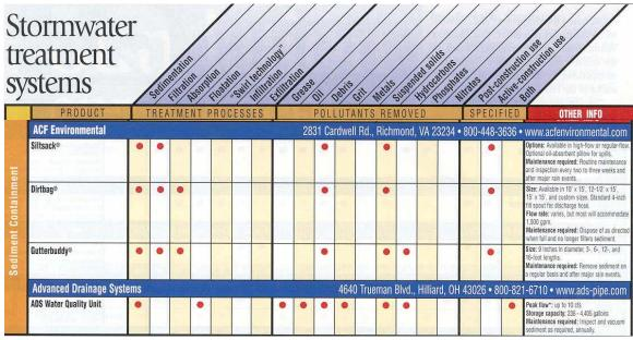
Figure 7.3c Available stormwater treatment systems (ASCE, 2003).
