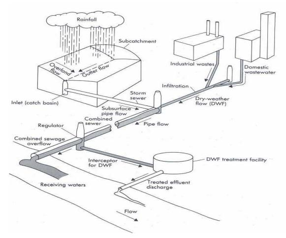
Figure 1.2 Combined urban drainage system (from Metcalf and Eddy et al., 1971).
