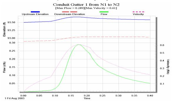
Figure D.29 Variation in flow and elevation with respect to time in the surface conduit Gutter 1 using rating curve.
