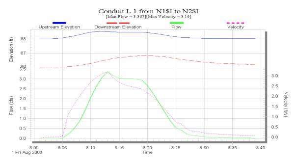
Figure D.23b Time series output of flow, velocity and elevation for conduit L-1 resulted from Extran layer of SWMM for a Maximum capacity of 3.0 cfs for inlet (**Time step for simulation 60 seconds**).
