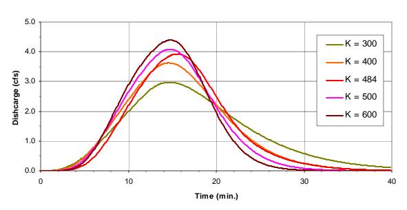
Comparison of Simulated Hydrographs in XP SWMM (SCS Method)
