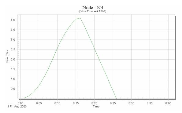
Figure D.18. SWMM output for Node-N4 solved in Runoff layer only.
