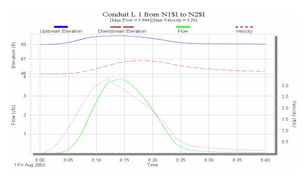
Figure D.27 Time series output of flow, velocity and elevation for conduit L-1 resulted from Extran layer of SWMM using rating curve as inlet restriction.
