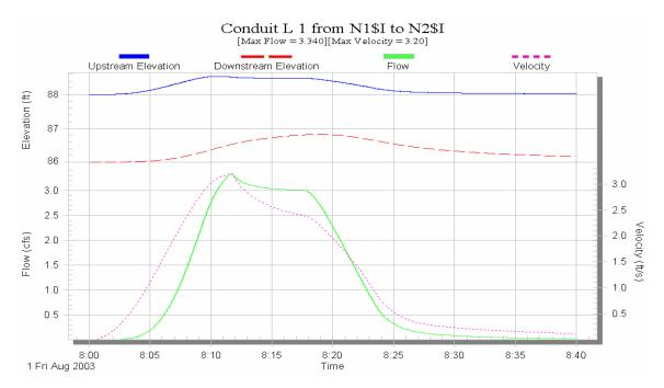
Figure D.23a Time series output of flow, velocity and elevation for conduit L-1 resulted from Extran layer of SWMM for a Maximum capacity of 3.0 cfs for inlet (**Time step for simulation 5 seconds**).
