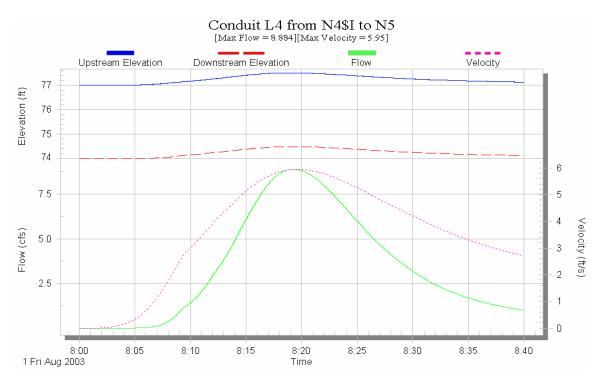
Figure D.38. Time series output from SWMM for conduit L-4.
