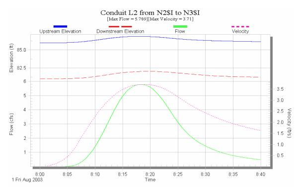
Figure D.28 Time series output of flow, velocity and elevation for conduit L-1 resulted from Extran layer of SWMM using rating curve as inlet restriction.
