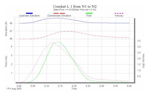
Figure D.20 Time series output of flow, velocity and elevation for conduit L-1 resulted from Extran layer of SWMM.
