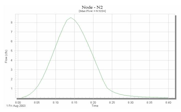
Figure D.14. Time series flow output by SWMM for Node-N2.
