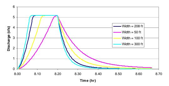
Figure D.6c. Sub-catchment hydrographs developed by Kinematic Wave Method with different basin widths.
