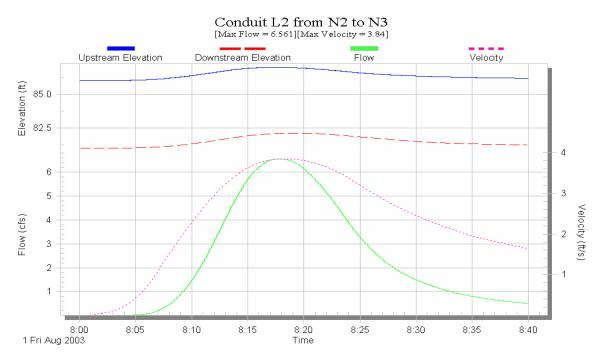
Figure D.21 Time series output of flow, velocity and elevation for conduit L-2 resulted from Extran layer of SWMM.
