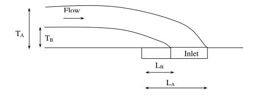
Figure 2.8 Characteristic spread  $T_A$  and  $T_B$  corresponding to inlet sizes  $L_A$  and  $L_B$  (after Fiuzat *et al.*, 2000)
