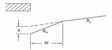
Figure 2.5. Depressed curb opening inlet (Brown et al., 2001).
