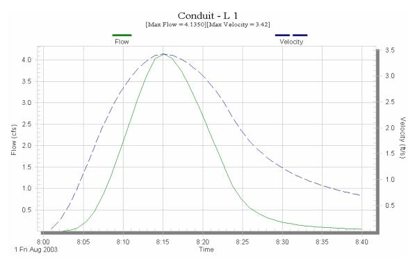
Figure 5.3. Time series plot of flows and velocity by SWMM for conduit L1.
