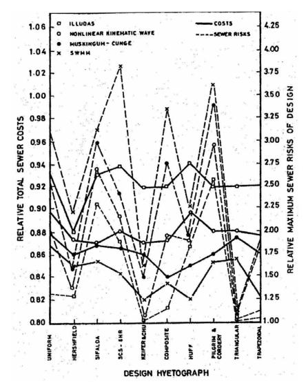
Figure 2.12 Effect of technique for routing flow through sewers on least-cost sewer system design (Nouh, 1987)
