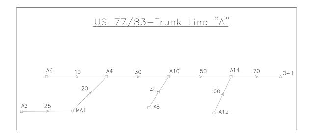
Figure 6.2. Layout of trunk line A of U.S. 77/83 under StormCAD.
