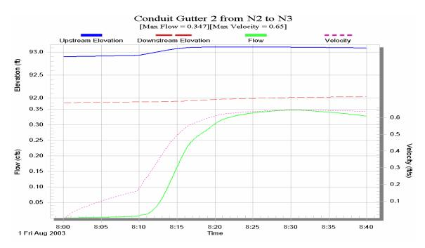
Figure D.26 Variation in flow and elevation with respect to time in the surface conduit Gutter 2.
