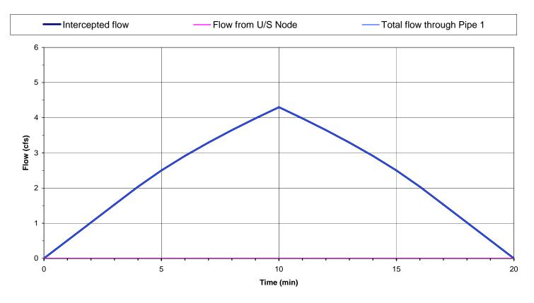
Figure C.2. Simulated subsurface flow components at the inlet I-1 (node 1) by using modified SPLIT program.
