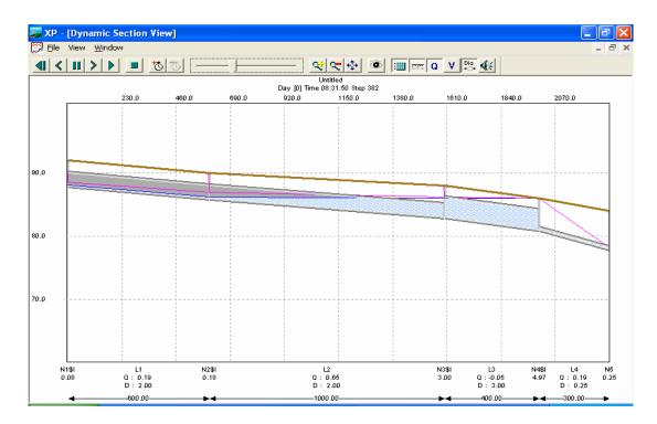
Figure 7.9 Dynamic section view of flooding occurred in Node 3 due to a smaller pipe size.
