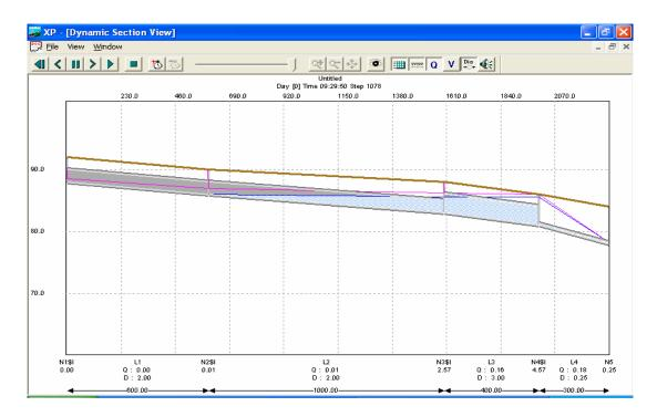
Figure 7.10 Dynamic section view at the end of simulation due to a smaller pipe size.
