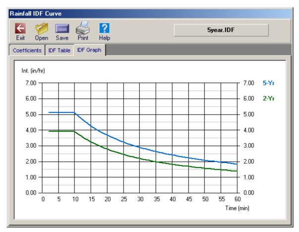
Figure B.2. Rainfall IDF Curve generated in Hydraflow
