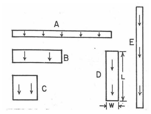
Figure D.6a. Different sub-catchment shapes to illustrate effect of sub-catchment width (Huber, 1988.)
