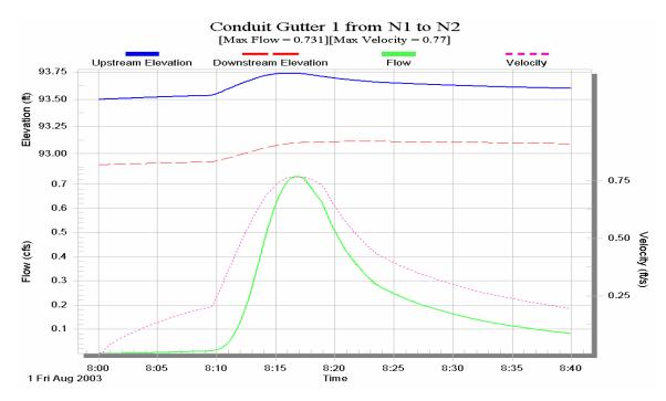
Figure D.25 Variation in flow and elevation with respect to time in the surface conduit Gutter 1.
