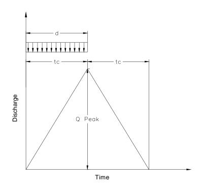
Figure 2.2(b) Hydrograph when duration of rainfall is equal to  $t_c$ .
