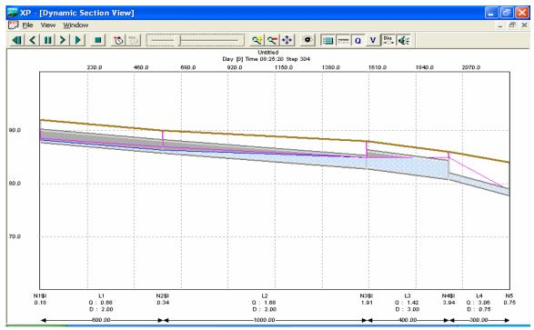
Figure 7.5 Storage capacity available and the head developed at time 8:25:20.
