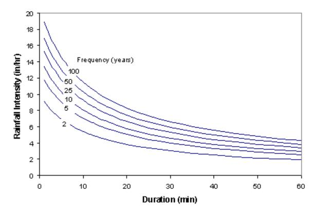
Figure 2.1 Intensity-Duration-Frequency (IDF) curves.
