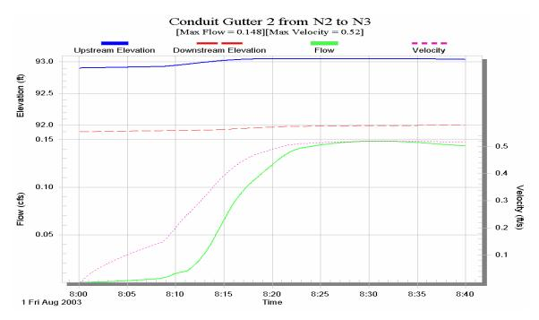
Figure D.30 Variation in flow and elevation with respect to time in the surface conduit Gutter 2 using rating curve.
