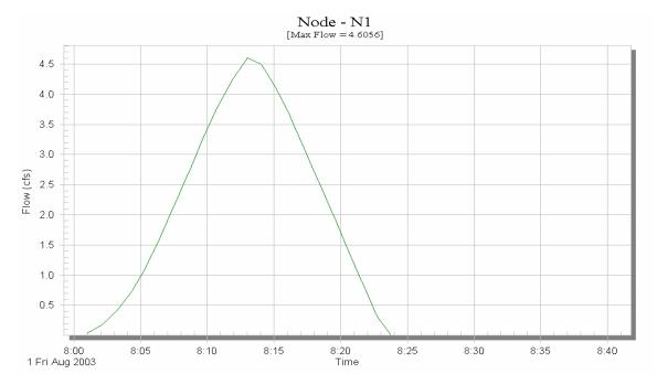
Figure 5.2. Hydrograph output of SWMM for Node N1.
