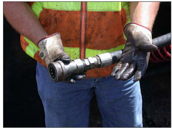
**Figure 5.7** Hydraulically-Controlled Trailer Ramp Systems Driven by the Power Take-Off/ Hydraulics from the Truck are Messy and Time-Consuming to Use
