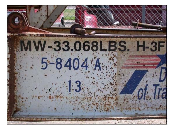
Figure 5.2 Payload Capacity is Frequently Incorrectly Marked, or Not Marked, on Trailers
