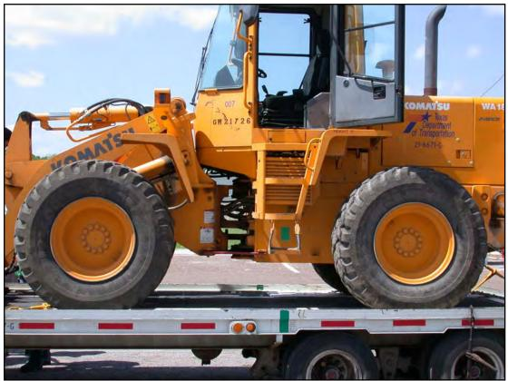
Figure 5.3 The "Green Line" on Trailers Does Not Always Provide an Accurate Alignment Mark for Proper Load Transfer
