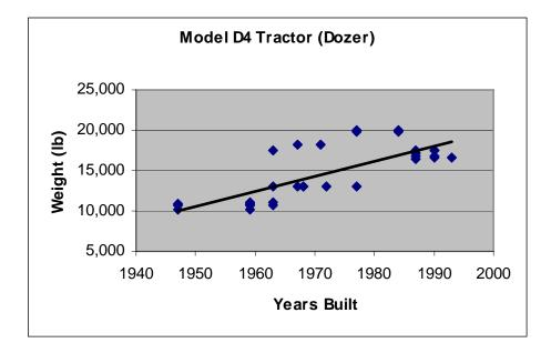
Figure 3.1 Increase in Weight in the Caterpillar Model D4 Tractor (Dozer) Over Time [17]
