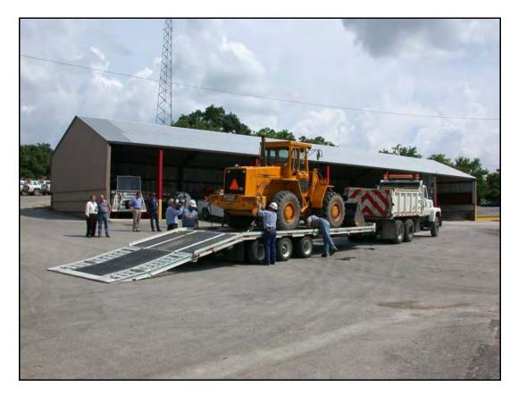
Figure 1.1 Common TxDOT Equipment Transport Practice: a Heavy Construction/ Maintenance Equipment Load (Front End Loader) Is Tied on a Tag-A-Long Trailer (Dovetail Style, Pintle Hitch) and Pulled by a 10 CY Dump Truck
