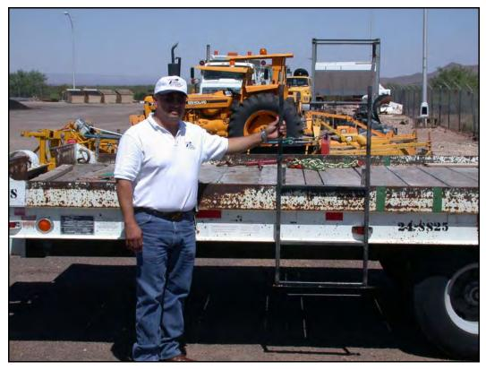
Figure 5.8 Storable Ladders on Trailers Help Provide for Worker Safety
