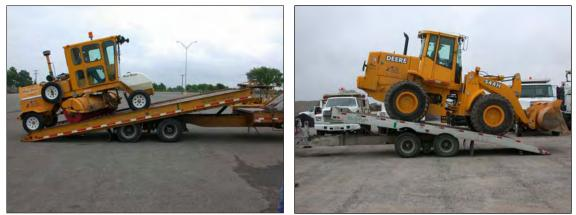
Figure 5.4 Tilt Deck Trailers are Suitable for Hauling Smaller Loads Such as the Broom (left) But Not the Very Large Loads Such as the Wheel Loader (right)
