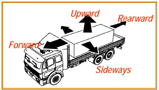
Figure 5.6 The New Cargo Securement Regulations Require Adequate Tie Down Sets to Resist Forward, Rearward, Sideways and Upward Forces
