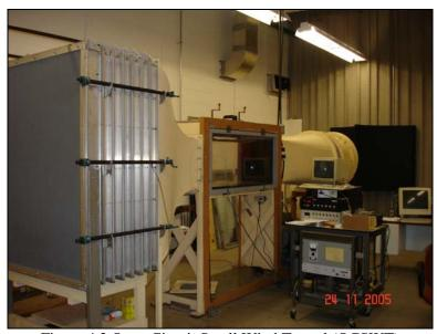
Figure 4.2 Open Circuit Small Wind Tunnel (OCSWT)
