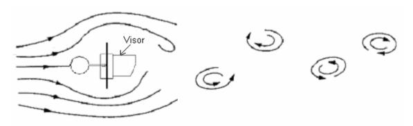
Figure 2.2 Vortex Shedding Acting on Cross-Section of Mast Arm with Traffic Signal
