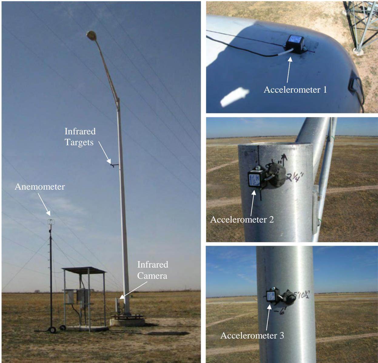
Figure 2 Forty feet lighting pole and the transducers used in monitoring
