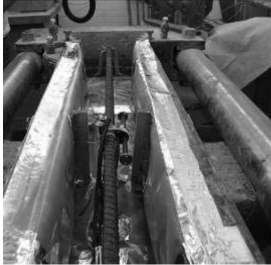
Figure 4.2: Horizontal cracking frame
