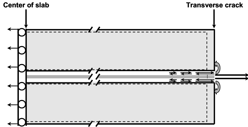
(a) Longitudinal restraint of steel on concrete subject to uniform temperature drop
