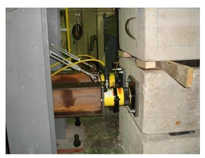
Figure 4.13 – Elevation View of Longitudinal Rams
