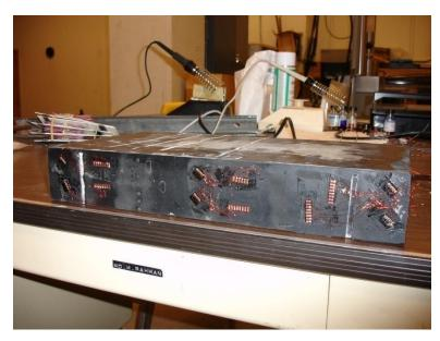
Figure 4.19 – Strain Gage Installed, 32-in. by 9-in. Bearing
