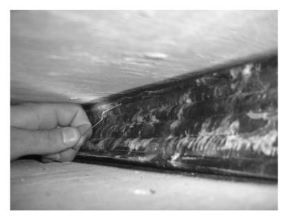
Figure 5.76 – Delamination of Elastomer
