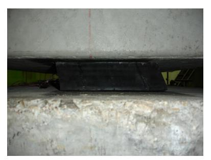
Figure 5.54 – Bearing Corner Undergoing Curling
