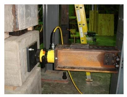
Figure 4.14 – Application of Transverse Load
