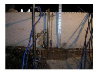
(a) Crackmeter for vertical movement measurements
