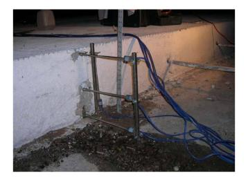
(a) Crackmeter for transverse movement measurements
