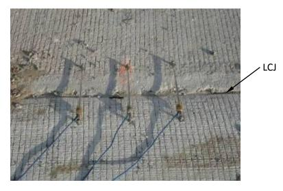
(a) Crackmeters installed at the surface across the LCJ in the tied section
