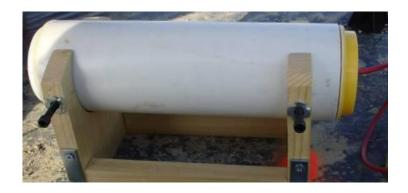
Figure 2.12: Non-stress cylinder installed in the field
