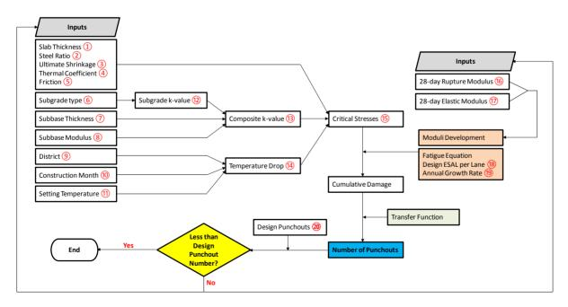
Figure 7.12 Architecture of TxCRCP-ME Software
