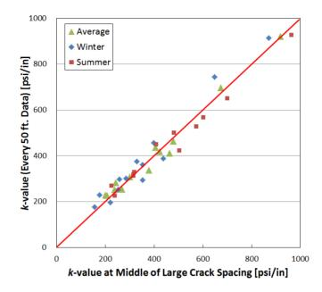
Figure 3.14 *k*-value Comparison between Deflection from Large Crack Spacing and Deflection from Every 50 ft
