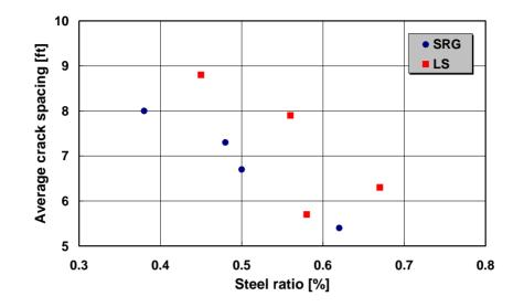
Figure 4.5 Correlation between Steel Percentage and Crack Spacing in BW 8 Section
