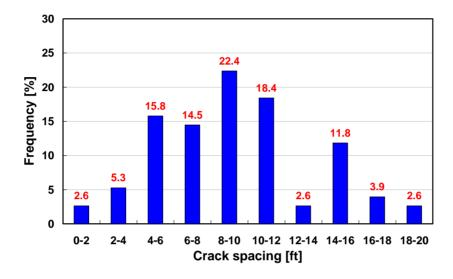
Figure 4.31 Crack Spacing Distributions in SPUR 330 Section in 2012
