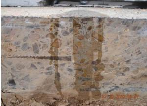
b. Tight crack width below the surface
