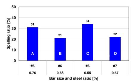
Figure 4.16 Spalling Ratio for SRG Sections
