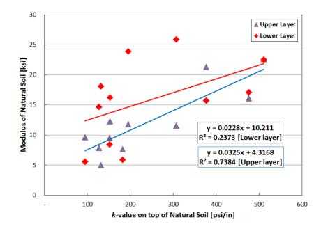
Figure 3.24 Comparison between k-value and Elastic Modulus on Natural Soil
