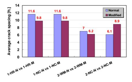
Figure 4.41 Effect of Batching Method on Average Crack Spacing
