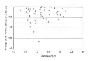
Figure 3.9 Correlation between crack spacing and LTE (Tayabji et al. 1999)
