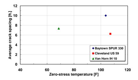
Figure 4.35 Average Transverse Crack Spacing vs. Zero-Stress Temperature
