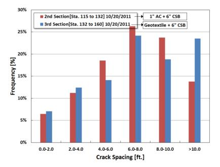
Figure 3.21 Transverse Cracking Pattern
