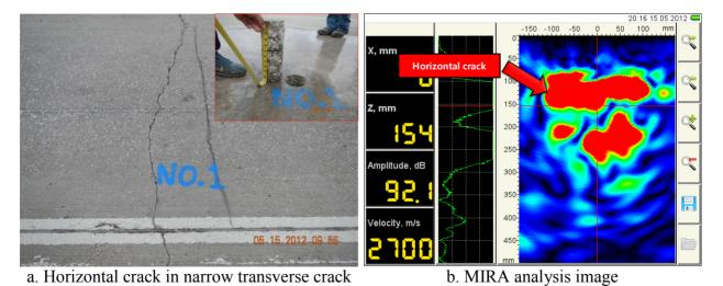
Figure 5.28 Horizontal Crack in Narrow Transverse Crack (IH 35 in the Laredo District)
