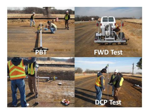
**Figure 3.23 Various Field Testings**
