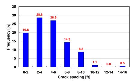
Figure 4.30 Crack Spacing Distributions in US 59 Cleveland Section in 2012
