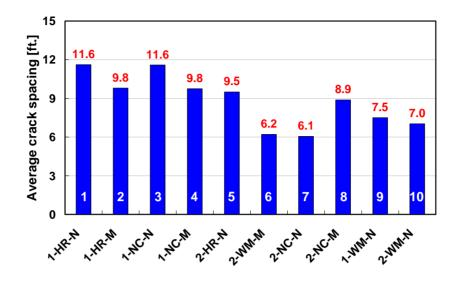
Figure 4.40 Average Crack Spacing Distributions for Pearland SH 288 Section
