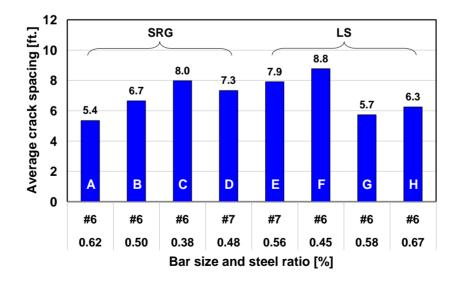
Figure 4.4 Average Crack Spacing of All Sections in BW 8 Frontage Road
