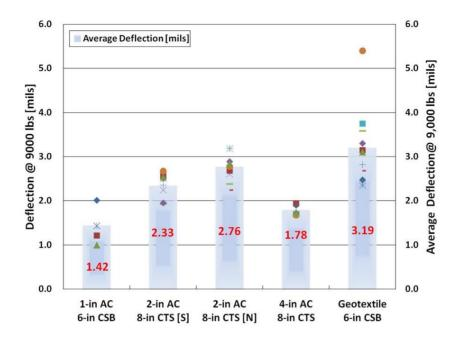
Figure 3.25 FWD Deflection Comparison with Different Base Types
