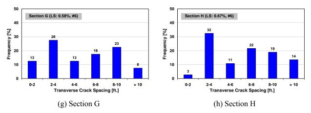
Figure C.1 Crack Spacing Distributions for Each Subsection of BW 8 Frontage Road Section
