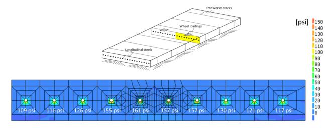
Figure 7.14 Principal Concrete Stresses under Wheel Loading
