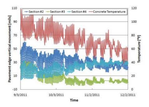
Figure 3.2 Pavement edge vertical movements
