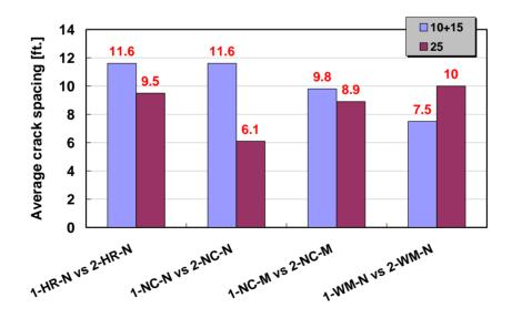
Figure 4.42 Effect of Fly Ash Replacement on Average Crack Spacing
