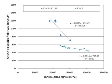
Figure 3.28 AREA k-value versus Combined Parameter for Two Base Types
