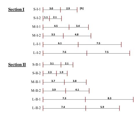
Figure C.5 Selected Cracks for FWD Testing in US290-3W
