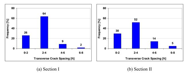
Figure 4.49 Crack Spacing Distribution of US 290-2E Section
