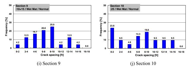
Figure C.3 Crack Spacing Distributions for Each Subsection of SH 288 Section
