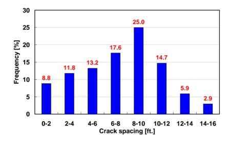
Figure 4.32 Crack Spacing Distributions in in Van Horn IH 10 Section
