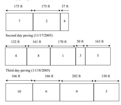
Figure 4.39 Configuration of Pearland SH 288 Section (Liu et al. 2009)
