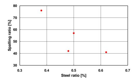
Figure 4.10 Relationship between Steel Percentage and Spalling Ratio for SRG Sections
