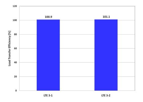
Figure 2.17 LTE in Upstream and Downstream of Punchout Slab
