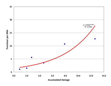
Figure 7.2 Transfer Hunction in TxDOT Research Project 0-5832
