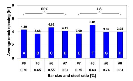
Figure 4.12 Average Crack Spacing in Various Sections
