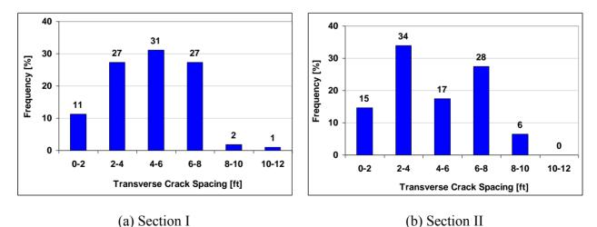
Figure 4.51 Crack Spacing Distribution of US290-3W Section
