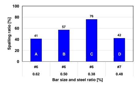
Figure 4.9 Spalling Ratio for SRG Sections
