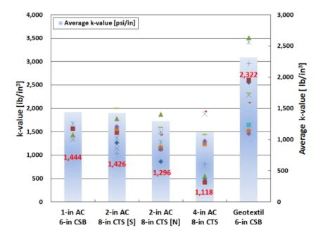
Figure 3.26 *k*-Value Comparison with Different Base Types
