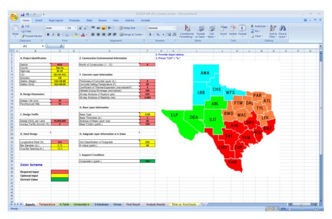
Figure 7.13 Input Screen of TxCRCP-ME
