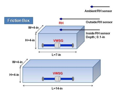
Figure 3.18 Concrete Prisms for Friction Evaluation
