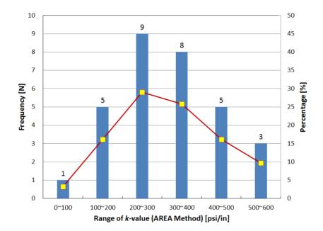
Figure 3.13 Backcalculated k-value Distribution of Level I Sections
