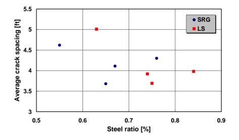
Figure 4.13 Relationship between Steel Percentage and Crack Spacing in SH 45 Section
