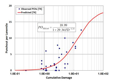
Figure 7.8 Transfer Function for TxCRCP-ME
