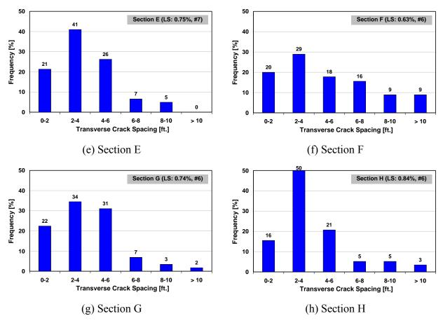
Figure C.2 Crack Spacing Distributions for Each Subsection of IH 45 Spring Creek Section
