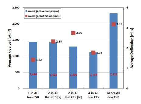
Figure 3.27 k-Value and Average Deflection with Different Base Types
