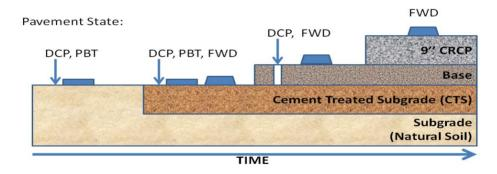
Figure 3.22 Field Testing
