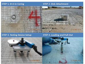
b. Bond strength testing procedure
