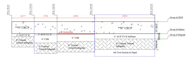
Figure 3.17 Test Section layout
