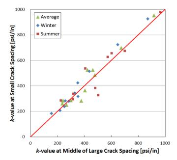
Figure 3.15 *k*-value Comparison between Deflection from Large Crack Spacing and Deflection from Small Crack Spacing
