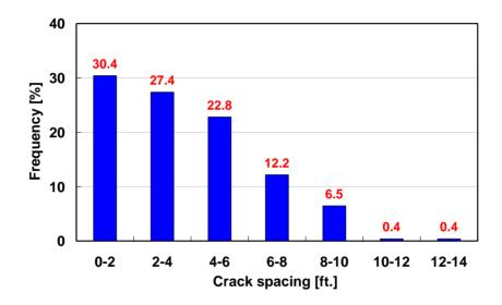
Figure 4.56 Crack Spacing Distributions for Waco IH 35 Section
