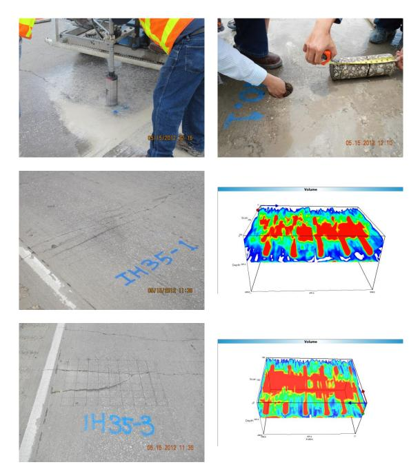
Figure D.7 IH 35 Pavement Evaluation in the Laredo District – Mira Test (05/15/2012)
