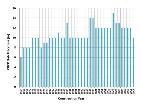
Figure 7.4 Slab Thickness Distribution vs. Construction Year
