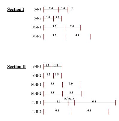
Figure C.4 Selected Cracks for FWD Testing in US290-2E
