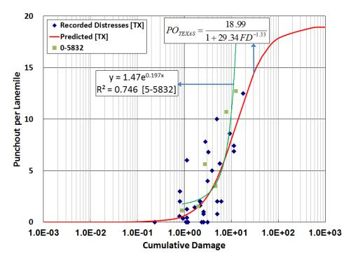
Figure B.8 Comparison of Transfer Function (0-5832 vs. 0-6274)
