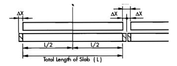
Figure 3.4 Relationship between total slab movement and total end movement (McCullough and Wu, 1992)
