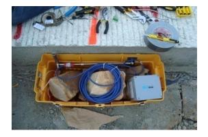
Figure 4.26 Setup of the datalogger and the crackmeter
