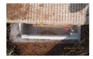
Figure 4.19 Crackmeter setup with protection box
