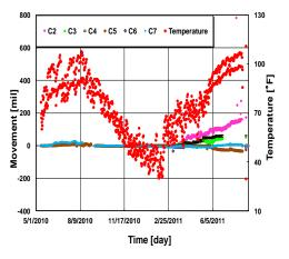
Figure 5.2 Concrete slab movement vs. concrete temperature for locations 1, 5, 7 and 8 (Refer to 4.17).
