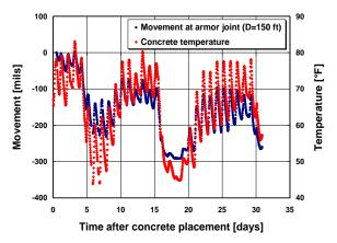
Figure 5.34 Concrete slab movement vs. concrete temperature
