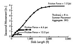
Figure 3.6 Typical seasonal movement in relation to slab length, and a comparison among three different friction forces (McCullough and Wu, 1992)
