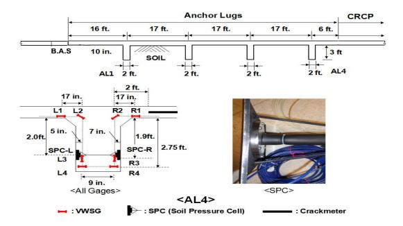
Figure 4.47 Section view of the anchor lugs, gages installation shown, jack out pressure cell
