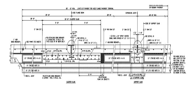
Figure 3.2 Wide-flange system (TxDOT, 2011)
