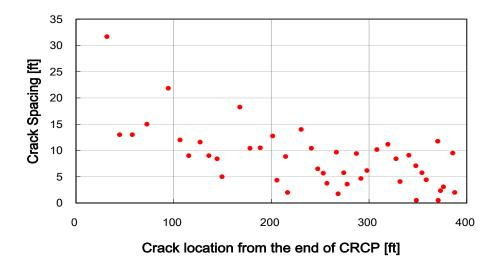
Figure 5.5 Crack spacing and crack location from the west end of the CRCP
