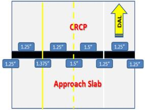
Figure 5.9 Joint widths at different locations of the expansion joint (East)
