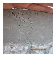
Figure 5.27 Location of the crack in AL4 at R1
