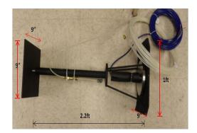
Figure 4.8 Jackout pressure cell assembly
