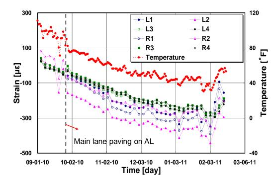
Figure 5.22 Concrete strains at different depths in AL1
