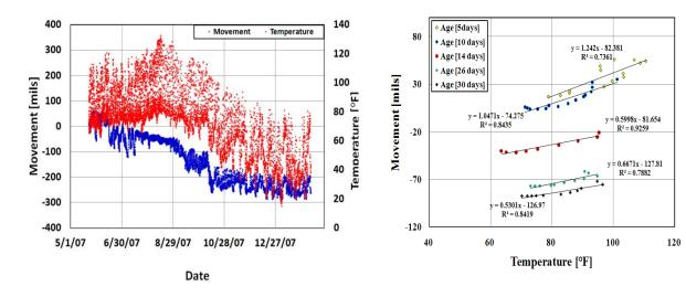
Figure 5.14 Slab movement vs. concrete temperature
