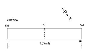
Figure 4.29 Location of crackmeter at the end of pavement near WF
