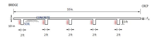
Figure 5.37 Example of CRCP with AL system
