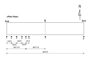
Figure 4.17 Location of eight crackmeters
