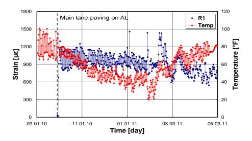
Figure 5.28 R1 movement vs. concrete temperature
