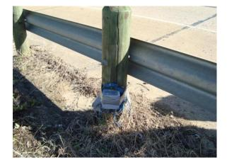
Figure 4.35 Datalogger installation
