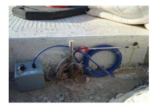
Figure 4.39 Installation of the crackmeter and the datalogger
