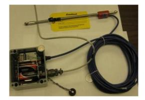
Figure 4.4 Wires from crackmeter connected to data logger
