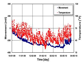
Figure 5.10 Concrete slab movement vs. concrete temperature
