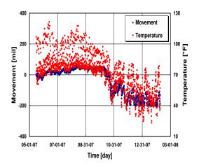
Figure 5.12 Slab movement vs. concrete temperature
