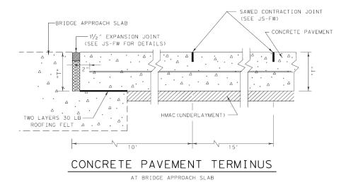
Figure 3.1 Typical expansion joint system (TxDOT, 2011)
