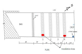
Figure 4.43 Installation location of all the gages
