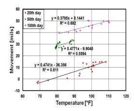
Figure 5.13 Daily movement rate of concrete slab
