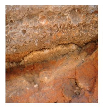
Figure 2.21 Undersealing material
