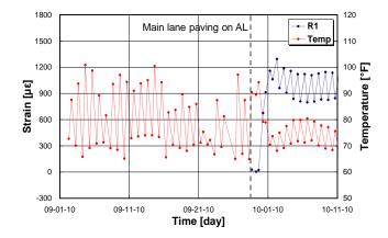
Figure 5.29 R1 movement vs. concrete temperature at the beginning of concrete placement
