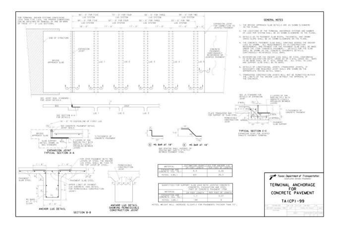
Figure 3.3 Anchor lug system (TxDOT, 2011)
