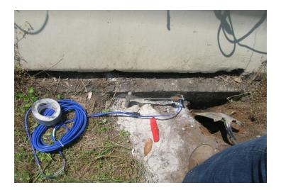
Figure 4.32 Crackmeter installed with the datalogger box
