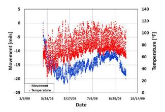
Figure 5.16 Concrete slab movement vs. concrete temperature
