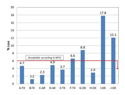
Figure 3.13 Unconfined (Canadian) Freeze and Thaw Loss of Aggregates
