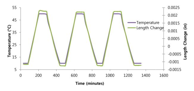
Figure 3.21 Three Cycles of Heating and Cooling and Change in Length for 4-in. x 7-in. Concrete Cylinder of B-TX
