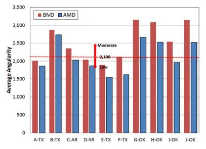
Figure 3.7 Average Angularity Before and After Micro-Deval
