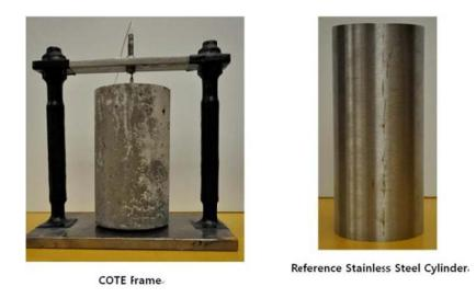
Figure 3.20 CoTE Frame and Reference Stainless Steel Cylinder
