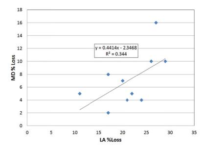
Figure 3.5 Comparison Between Micro-Deval and L.A. Abrasion
