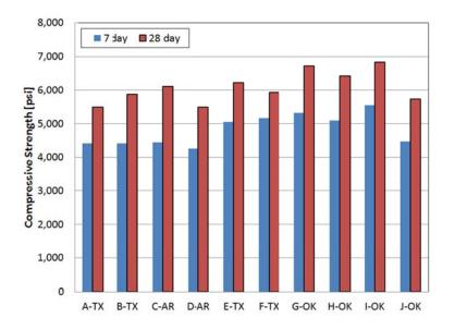
Figure 3.15 Seven-Day and 28-Day Compressive Strength of Concrete
