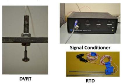
Figure 3.18 Various Components of CoTE Setup
