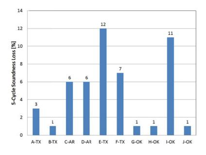
Figure 3.2 Sulfate Soundness of Aggregates
