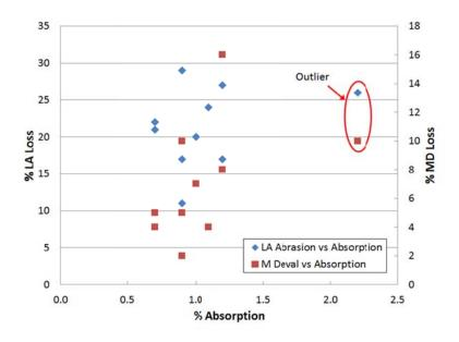
Figure 3.6 Relation Between Absorption vs. %LA and %MD Losses
