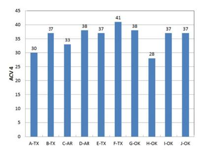
Figure 3.14 Aggregate Crushing Value
