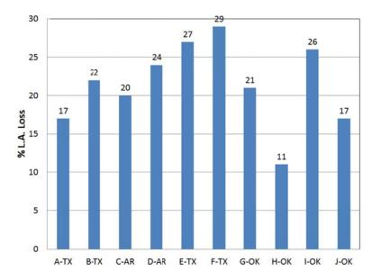
Figure 3.1 L.A. Abrasion Loss for Aggregates
