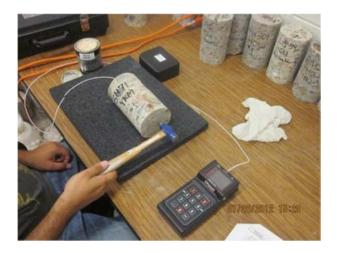
**Figure 2.21 Resonant Frequency Test**
