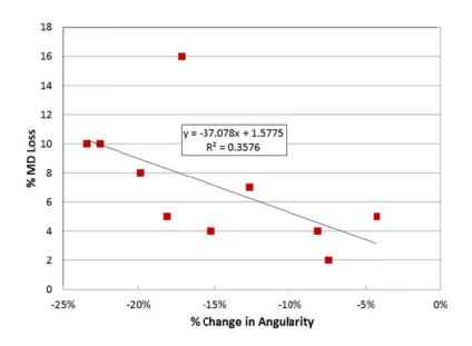
Figure 3.9 Comparison Between % Change in Angularity and % Micro-Deval Loss
