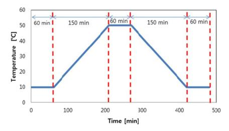
Figure 3.19 One Cycle of Heating and Cooling
