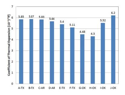
Figure 3.22 CoTE for Concrete Specimens Older than 28 Days
