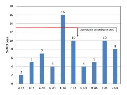
Figure 3.4 Micro-Deval Loss for Aggregates
