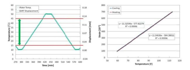
(a) Temperature Range for CoTE Calculation (b) CoTE value of Calibration Cylinder Figure 2.20 CoTE Test for Reference Cylinder
