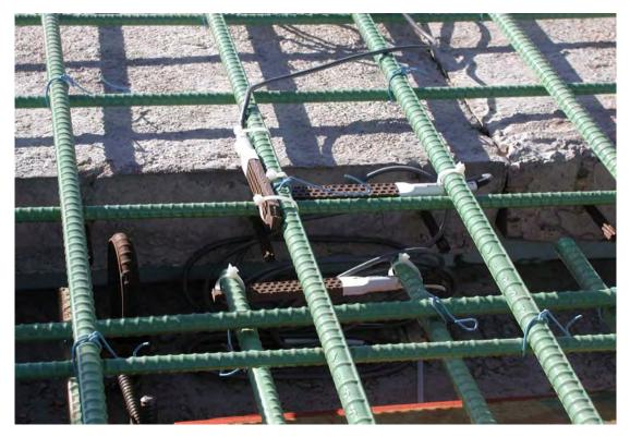
Figure 3.4. Embedded Concrete Strain Gauges Over an Interior Beam
