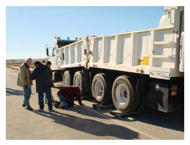
Figure 4.3 Crack Measuring with TxDOT Dump Trucks in a Back-to-back Load Case Photograph: Courtesy of Alvin Gutierrez, FHWA
