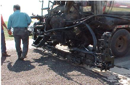
Figure 3. Distributor Spray Bar
