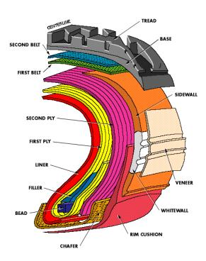
Figure 2.4 Radial Passenger Tire Construction (Cooper Tire & Rubber Company 1999)
