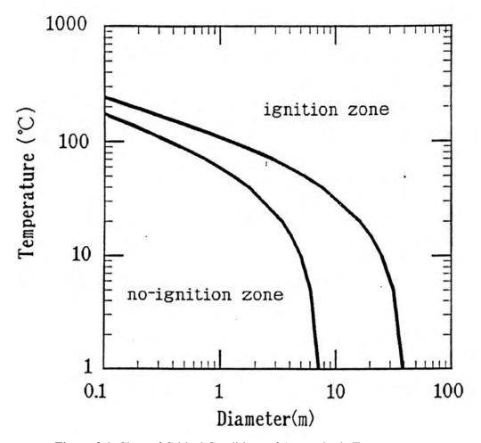
**Figure 3.1** Chart of Critical Conditions of Atmospheric Temperature and Sample Size for Spontaneous Combustion of Used Tire Chips for Tire Chip Density of 400 kg/m<sup>3</sup> (Sugawa 1993)
