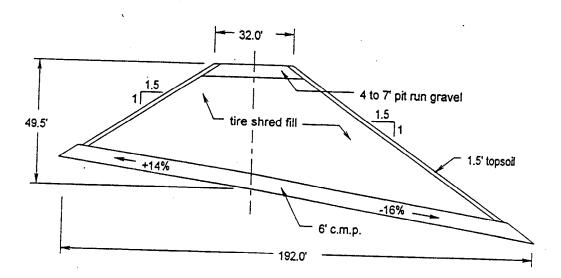
Figure 4.2 Cross Section of Tire Fill in Garfield Co., Washington (Humphrey 1996)
