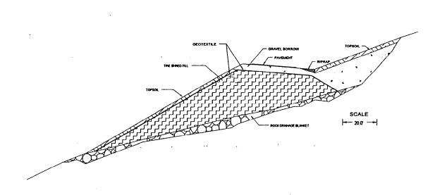
**Figure 4.1** Cross Section of Tire Fill in Ilwaco, Washington (Humphrey 1996)
