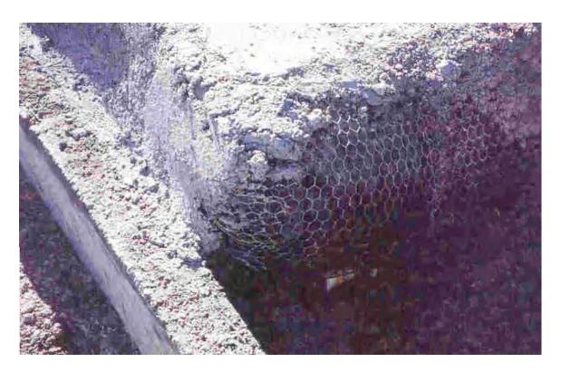
**Figure 5.9** A Tire Bale Partly Encapsulated in Cement (NMED 1999)
