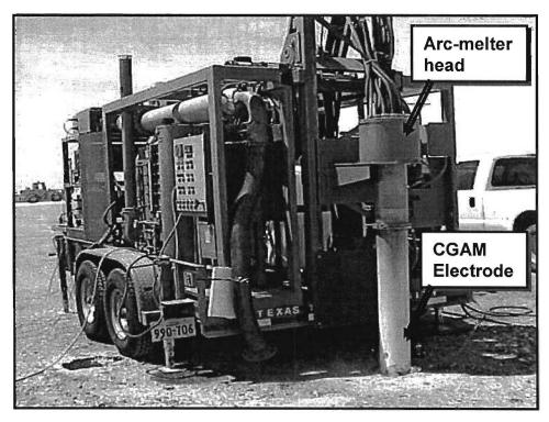
Figure 1. Mobile, Trailer-Mounted SOVIT System
