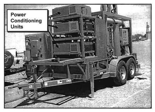
Figure 3. Power Conditioning Unit
