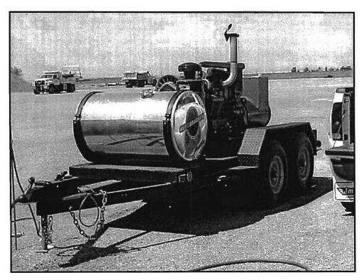
Figure 2. Electric Power Generator Used with SOVIT
