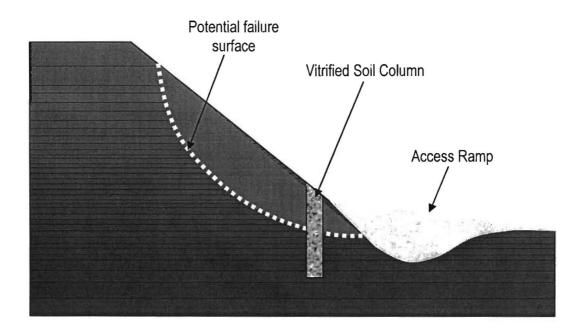
Figure 10. Use of In-situ Soil Vitrification for Slope Stabilization
