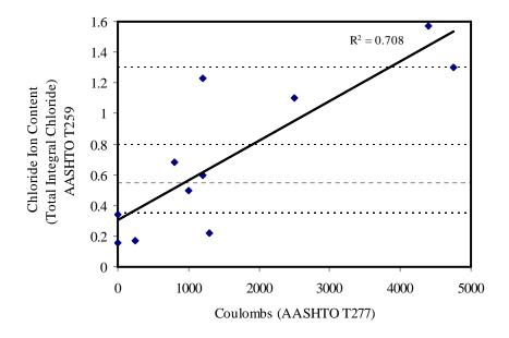
Figure 2.7 Correlation Data of ASTM C1202 Document (Whiting, 1981)
