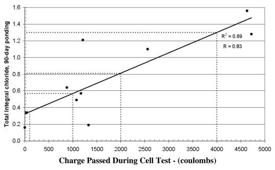
Figure 1.3 RCPT and Integral Chloride Correlation (Whiting 1981)
