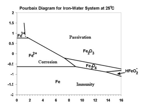
**Figure 2.1** Pourbaix Diagram for the FeO-H<sub>2</sub>O System at  $77^{\circ}F(25^{\circ}C)$  for  $10^{-6}M$  Activities of All Metal Ions (Pourbaix (1976)
