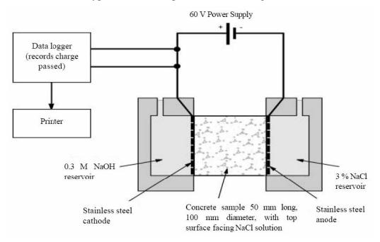
Figure 1.1 Typical RCPT Setup (Stanish, K.D. et al., 1997)
