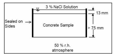
Figure 1.2 Ponding Test Setup (Stanish, K.D. et al., 1997)
