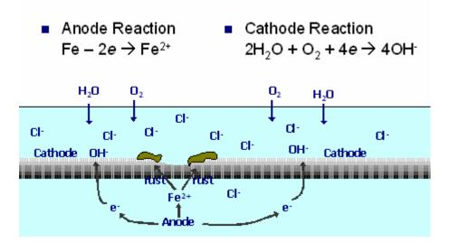
Figure 2.3 Mechanism of Corrosion of Steel in Concrete (Mehta 1993)
