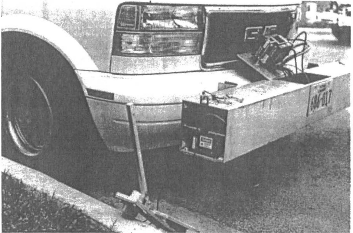
Figure 6.10: Sensor Bar Mounted to the Profiler/Rubar Vehicle.
