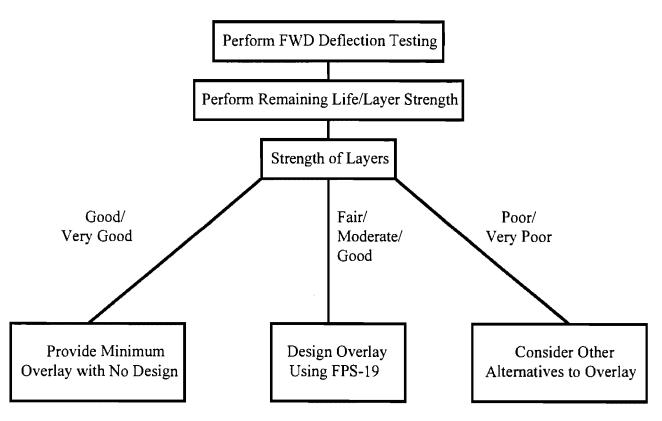
FIG. D-1. Schematic Diagram of TxDOT Pavement Rehabilitation Design Process
