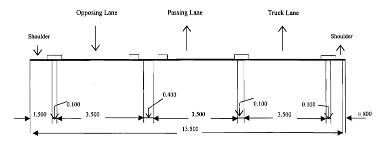
Figure 2-4: Three Lane Highway Cross Section in Mexico
