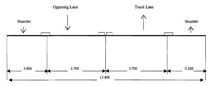
Figure 2-1: Current Two-Lane Rural Highway Cross-section
