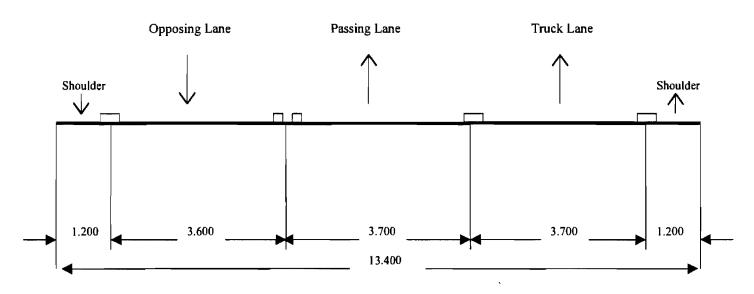
Figure 2-2: Three Lane Highway Cross Section in Canada
