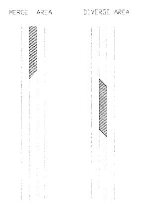
Figure B-1: Type A Design with Continuous Interior Alternating Passing Lane
