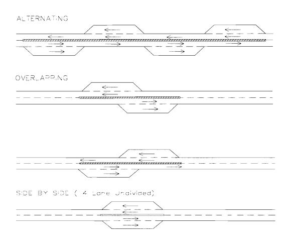
Figure B-3: Type C Design with Overlapping Passing Sections
