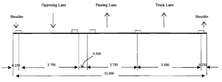
Figure 2-3: Three Lane Highway Cross Section in Germany
