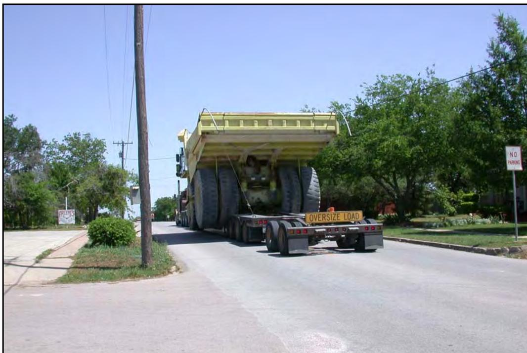
**FIG. 4.23.** An Example of Oversize Traffic Taking Its Half (More than Half) Out of the Middle.
