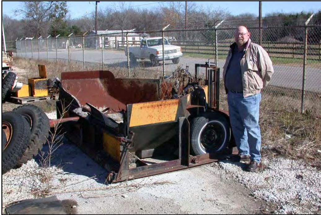
**FIG. 7.8** Drag Box; Tow-Behind, Used for Delivering Material to the Left, Center, or Right Side of Pavement, Waco District (see Waco District Profile, Photo 8)
