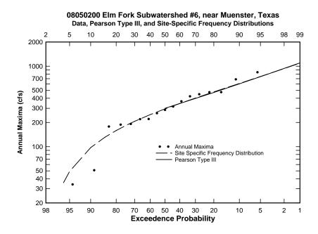
Figure C.16: Flood frequency curve for USGS station 08050200
