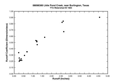
Figure D.10: Plot of runoff coefficient versus runoff depth for watershed 08098300
