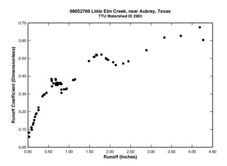
Figure D.18: Plot of runoff coefficient versus runoff depth for watershed 08052700
