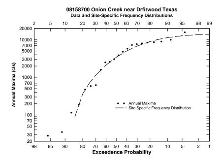
Figure C.6: Flood frequency curve for USGS station 08158700
