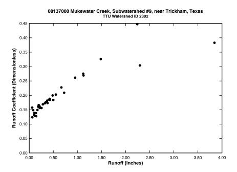
Figure D.12: Plot of runoff coefficient versus runoff depth for watershed 08137000
