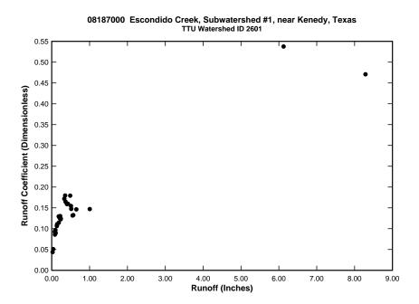
Figure D.14: Plot of runoff coefficient versus runoff depth for watershed 08187000
