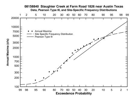
Figure C.7: Flood frequency curve for USGS station 08158840
