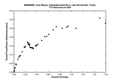
Figure D.11: Plot of runoff coefficient versus runoff depth for watershed 08096800
