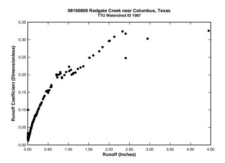
Figure D.3: Plot of runoff coefficient versus runoff depth for watershed 08160800
