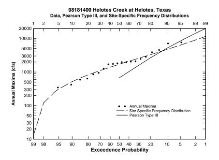
Figure C.9: Flood frequency curve for USGS station 08181400
