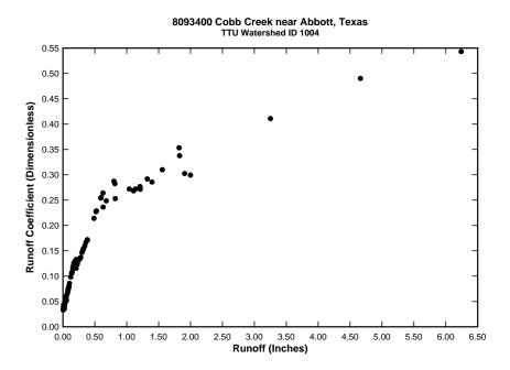
Figure D.2: Plot of runoff coefficient versus runoff depth for watershed 08093400
