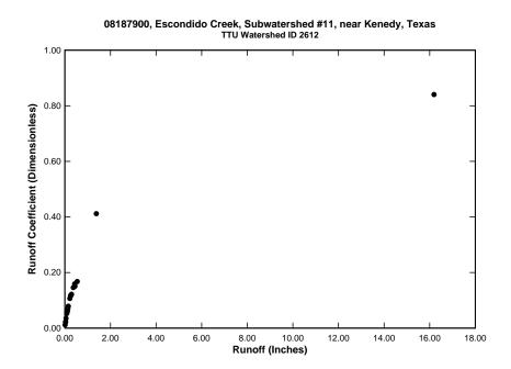
Figure D.15: Plot of runoff coefficient versus runoff depth for watershed 08187900
