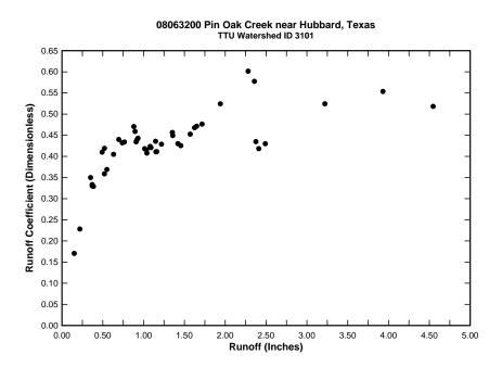
Figure D.20: Plot of runoff coefficient versus runoff depth for watershed 08063200
