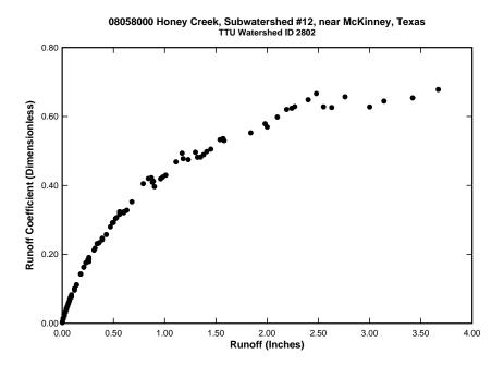
Figure D.17: Plot of runoff coefficient versus runoff depth for watershed 08058000
