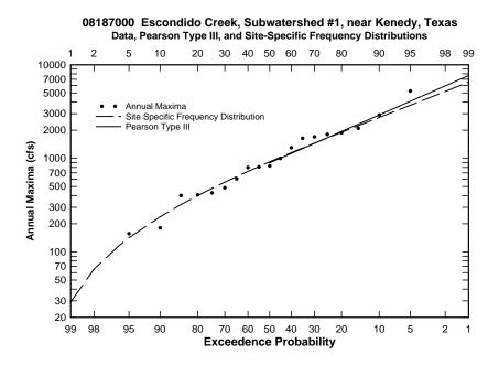
Figure C.14: Flood frequency curve for USGS station 08187000
