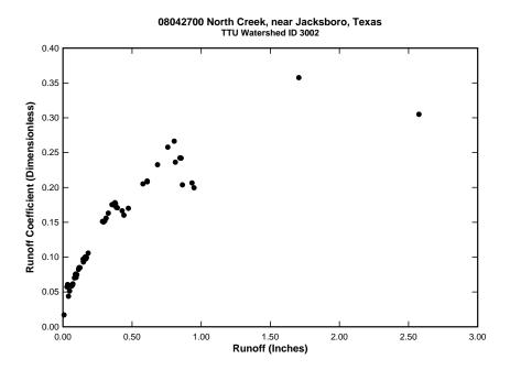
Figure D.19: Plot of runoff coefficient versus runoff depth for watershed 08042700
