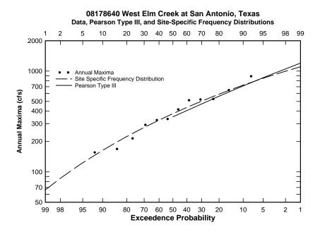
Figure C.8: Flood frequency curve for USGS station 08178640
