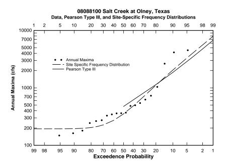
Figure C.1: Flood frequency curve for USGS station 08088100
