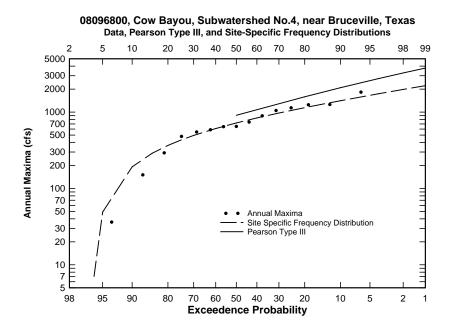
Figure C.11: Flood frequency curve for USGS station 08096800
