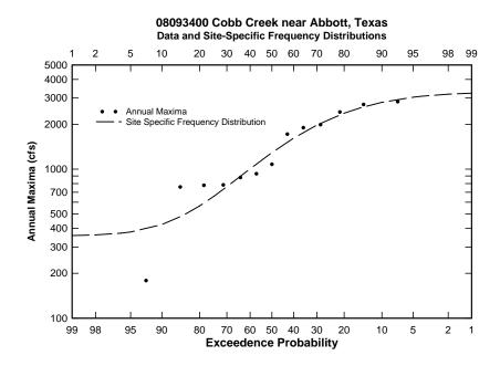
Figure C.2: Flood frequency curve for USGS station 08093400
