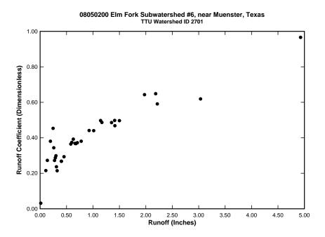
Figure D.16: Plot of runoff coefficient versus runoff depth for watershed 08050200
