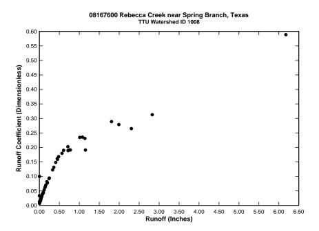
Figure D.4: Plot of runoff coefficient versus runoff depth for watershed 08167600
