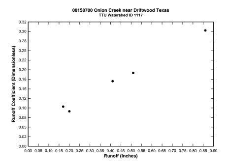
Figure D.6: Plot of runoff coefficient versus runoff depth for watershed 08158700
