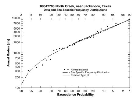
Figure C.19: Flood frequency curve for USGS station 08042700
