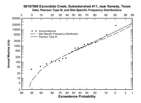
Figure C.15: Flood frequency curve for USGS station 08187900
