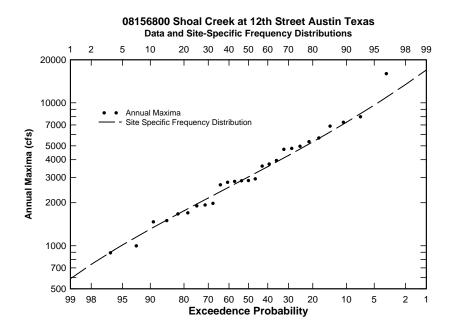
Figure C.5: Flood frequency curve for USGS station 08156800
