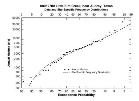
Figure C.18: Flood frequency curve for USGS station 08052700
