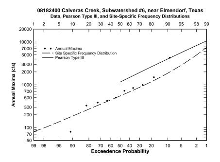
Figure C.13: Flood frequency curve for USGS station 08182400
