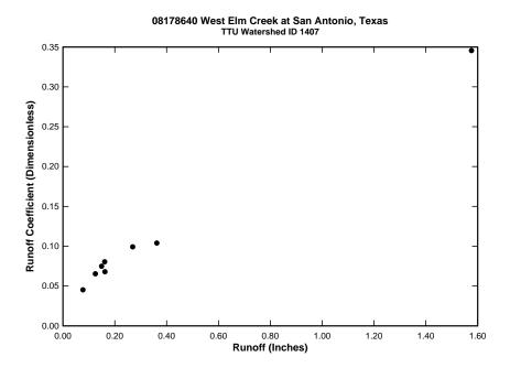
Figure D.8: Plot of runoff coefficient versus runoff depth for watershed 08178640
