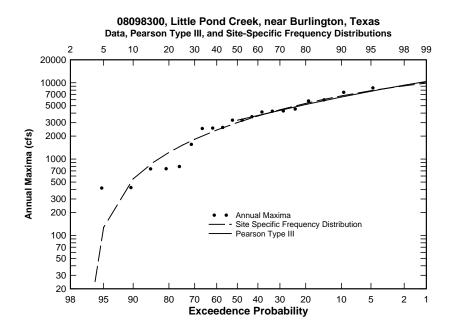
Figure C.10: Flood frequency curve for USGS station 08098300
