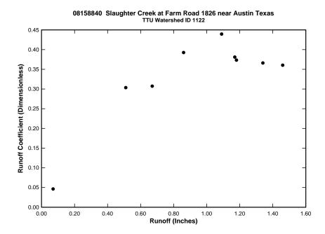
Figure D.7: Plot of runoff coefficient versus runoff depth for watershed 08158840
