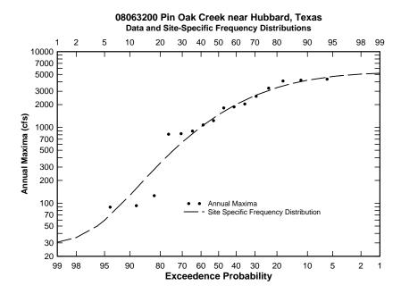
Figure C.20: Flood frequency curve for USGS station 08063200
