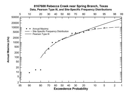
Figure C.4: Flood frequency curve for USGS station 08167600
