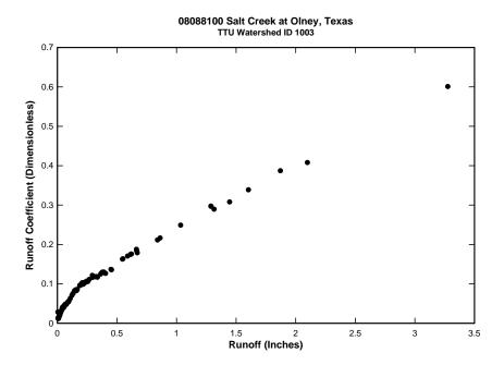
Figure D.1: Plot of runoff coefficient versus runoff depth for watershed 08088100
