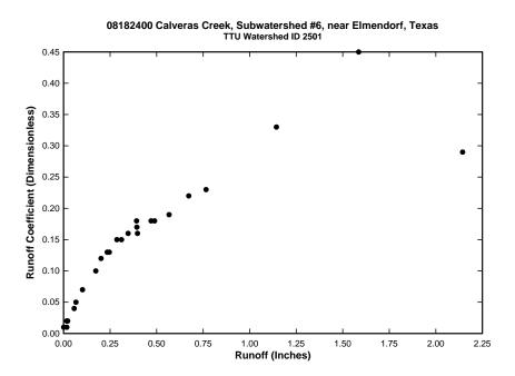
Figure D.13: Plot of runoff coefficient versus runoff depth for watershed 08182400
