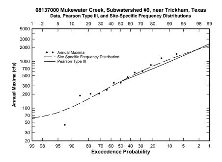
Figure C.12: Flood frequency curve for USGS station 08137000
