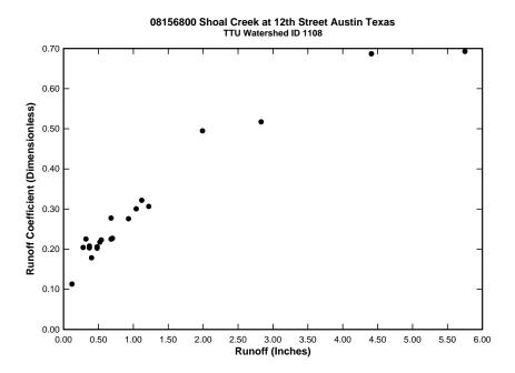
Figure D.5: Plot of runoff coefficient versus runoff depth for watershed 08156800
