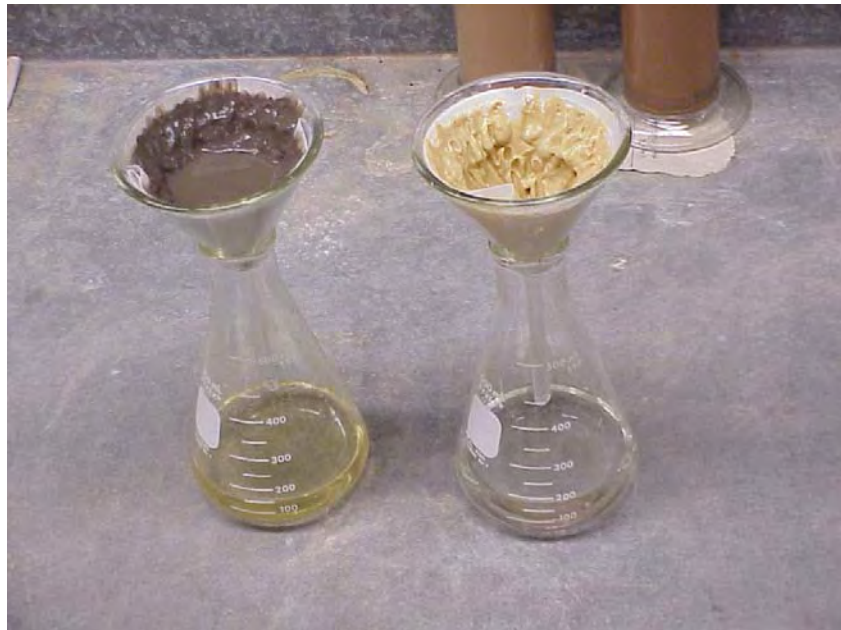
Figure 4.4 Filtering Process in Soil Sulfate Content Testing
