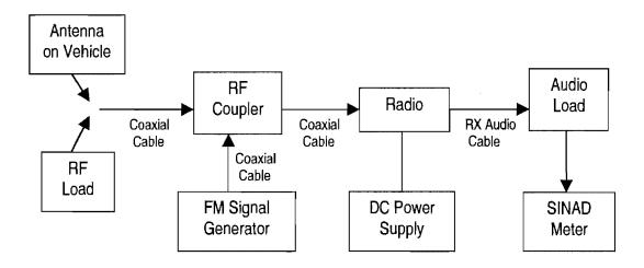
Figure 3. Setup for Site Qualification and Egress Compliance Test
