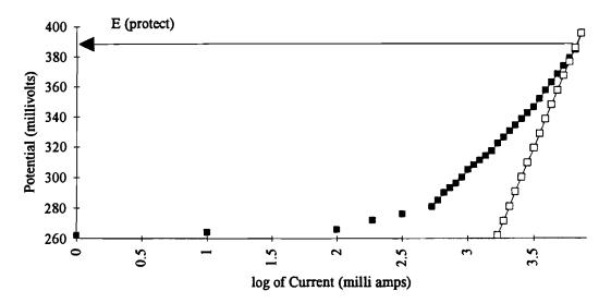
Figure 6. Typical Tafel Diagram for Big Spring Bridge (Smith, 1990)
