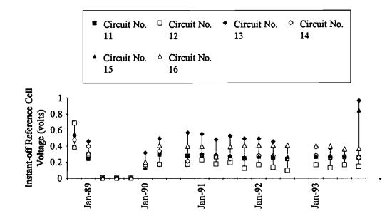
Figure 32. Instant-off Reference Cell Voltage, Quarterly Averages - Sprayed Zinc Anode
