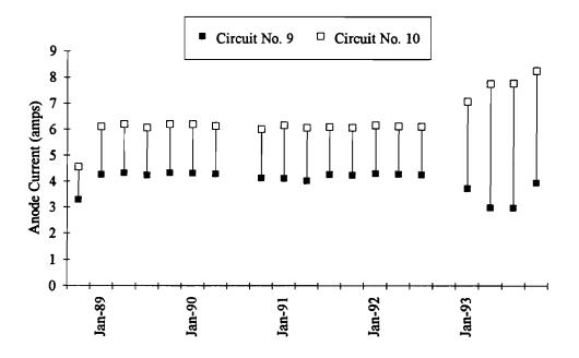
Figure 22. Anode Current, Quarterly Averages - Carbon Strand Anode
