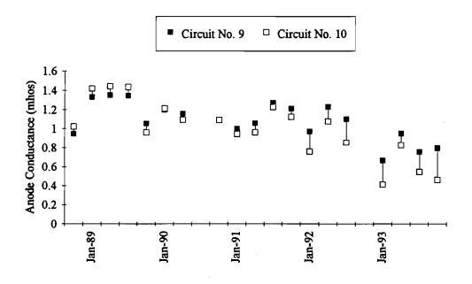
Figure 24. Anode Conductance, Quarterly Averages - Carbon Strand Anode
