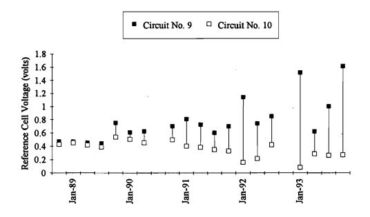
Figure 25. Reference Cell Voltage, Quarterly Averages - Carbon Strand Anode
