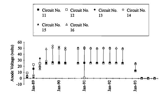
Figure 29. Anode Voltage, Quarterly Averages - Sprayed Zinc Anode
