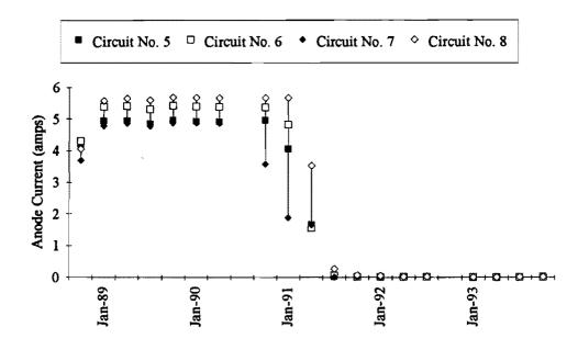
Figure 16. Anode Current, Quarterly Averages - Conductive Polymer Anode
