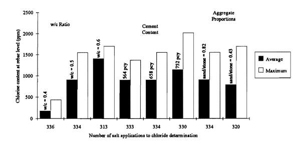
Figure 3. Effect of Mix Design Parameters (Clear, 1974)
