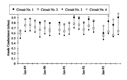
Figure 12. Anode Conductance, Quarterly Averages - Titanium Mesh Anode
