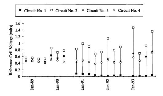
Figure 13. Reference Cell Voltage, Quarterly Averages - Titanium Mesh Anode
