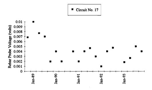
Figure 39. Rebar Probe Voltage, Quarterly Averages - Conductive Paint Anode
