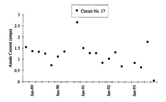
Figure 34. Anode Current, Quarterly Averages - Conductive Paint Anode
