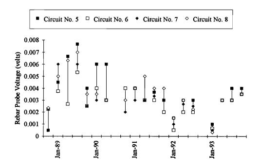
Figure 21. Rebar Probe Voltage, Quarterly Averages - Conductive Polymer Anode
