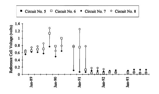
Figure 19. Reference Cell Voltage, Quarterly Averages - Conductive Polymer Anode
