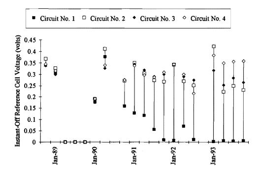
Figure 14. Instant-off Reference Cell Voltage, Quarterly Averages - Titanium Mesh Anode
