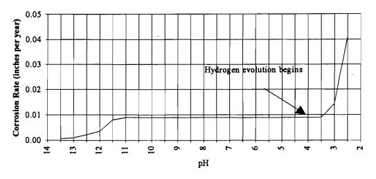
One inch = 2.54 cm Figure 2. Effect of pH on Corrosion of Iron in Aerated Soft Water at Room Temperature (Uhlig, 1985)
