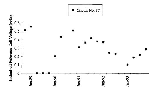
Figure 38. Instant-off Reference Cell Voltage, Quarterly Averages - Conductive Paint Anode
