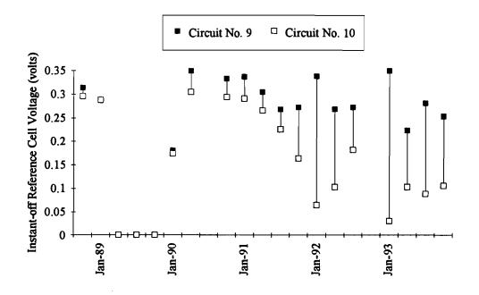
Figure 26. Instant-off Reference Cell Voltage, Quarterly Averages - Carbon Strand Anode
