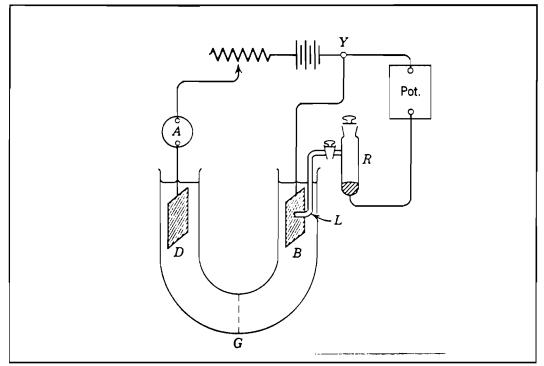
Figure 5. Cell for Measuring Polarization (Uhlig, 1985)
