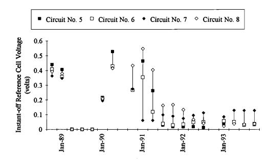
Figure 20. Instant-off Reference Cell Voltage, Quarterly Averages - Conductive Polymer Anode
