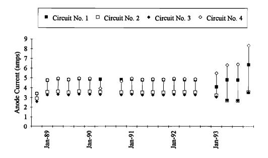
Figure 10. Anode Current, Quarterly Averages - Titanium Mesh Anode
