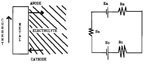
Figure 1. Simple Cell and Equivalent Circuit (Morgan, 1959)
