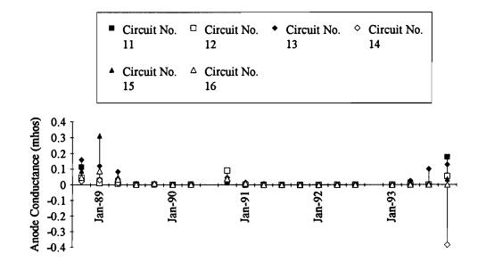
Figure 30. Anode Conductance, Quarterly Averages - Sprayed Zinc Anode
