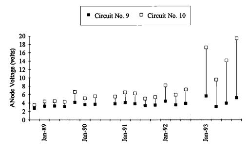
Figure 23. Anode Voltage, Quarterly Averages - Carbon Strand Anode
