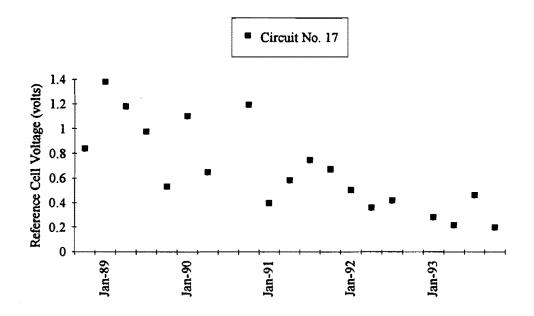
Figure 37. Reference Cell Voltage, Quarterly Averages - Conductive Paint Anode
