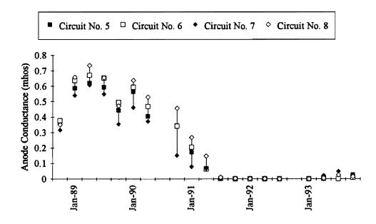
Figure 18. Anode Conductance, Quarterly Averages - Conductive Polymer Anode
