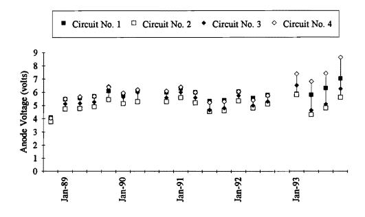
Figure 11. Anode Voltage, Quarterly Averages - Titanium Mesh Anode
