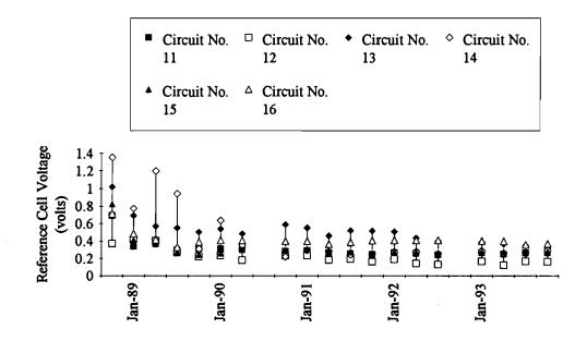
Figure 31. Reference Cell Voltage, Quarterly Averages - Sprayed Zinc Anode
