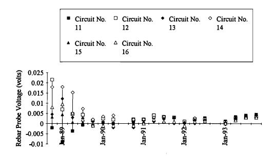
Figure 33. Rebar Probe Voltage, Quarterly Averages - Sprayed Zinc Anode
