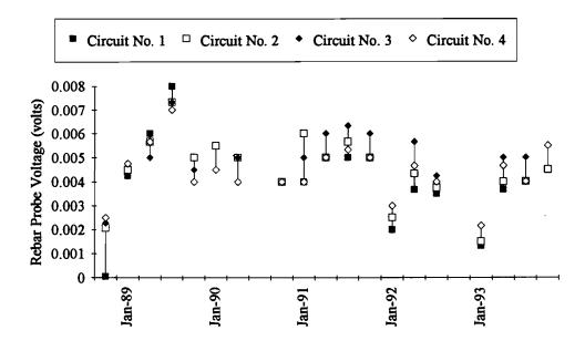
Figure 15. Rebar Probe Voltage, Quarterly Averages - Titanium Mesh Anode
