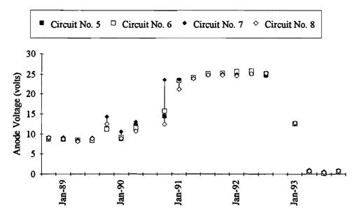
Figure 17. Anode Voltage, Quarterly Averages - Conductive Polymer Anode
