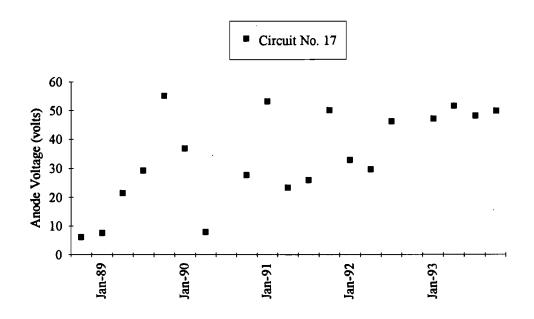
Figure 35. Anode Voltage, Quarterly Averages - Conductive Paint Anode
