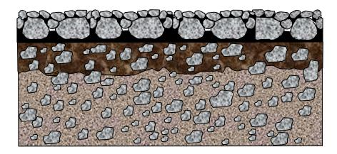
Figure 2.3 Schematic of a Typical Two-Course AST
