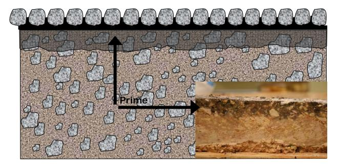
Figure 4.5 Schematic of Prime Coat Penetration into Base
