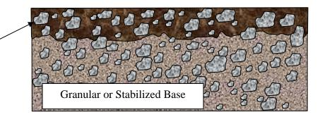
Figure 2.1 Schematic of Prime Coat Penetration into Base Layer
