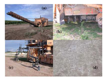
Figure 5.2 Trimming Machine Used in Base Finishing (a) Machine with Excess Material Loading Conveyor (b) Cutting Blades, (c) Guide Roller Assembly and (d) Finished Base Surface After Rolling
