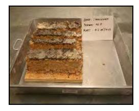
Figure 3.4 Cut Specimen Beams
