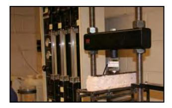
Figure 3.5 Flexural Strength Testing Arrangement
