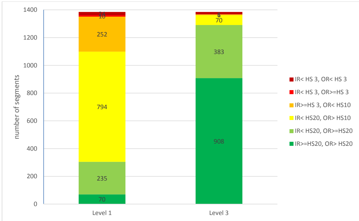
Figure 10.6. Level 1 versus Level 3 Load Rating for Load Rated Segments ( n = 1,385 )
