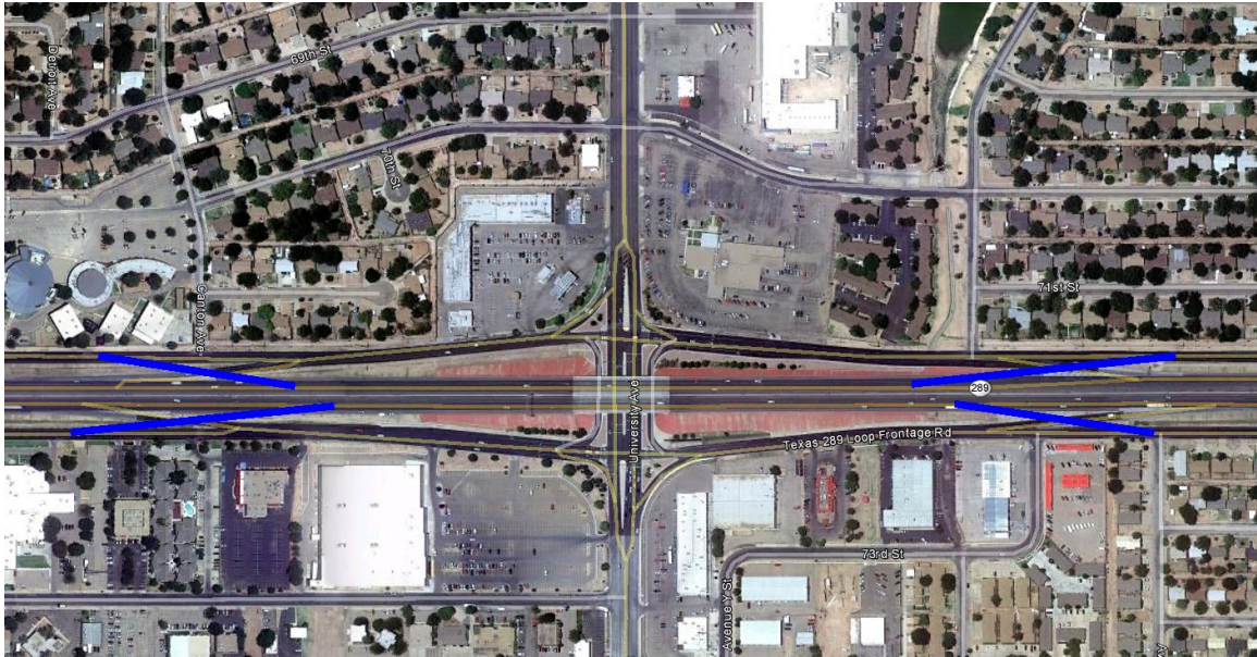
Figure 3-3: Proposed X Type Ramp Design at the Interchange of University Avenue and South Loop 289
