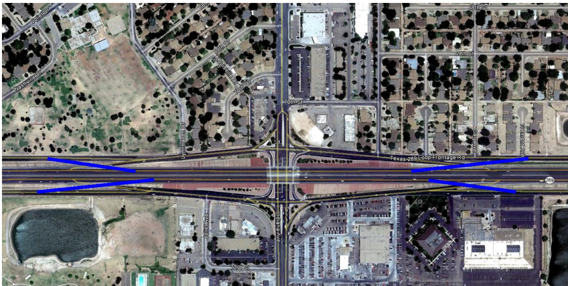
Figure 3-2: Proposed X Type Ramp Design at the Interchange of Indiana Avenue and South Loop 289
