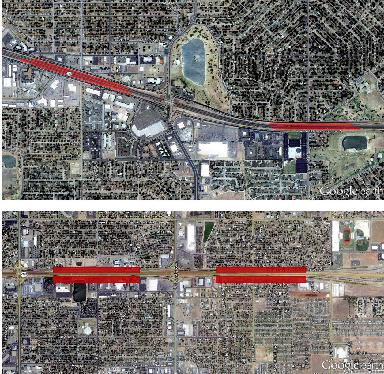
Figure 1-4: Alternative #1: Auxiliary Lane Addition
