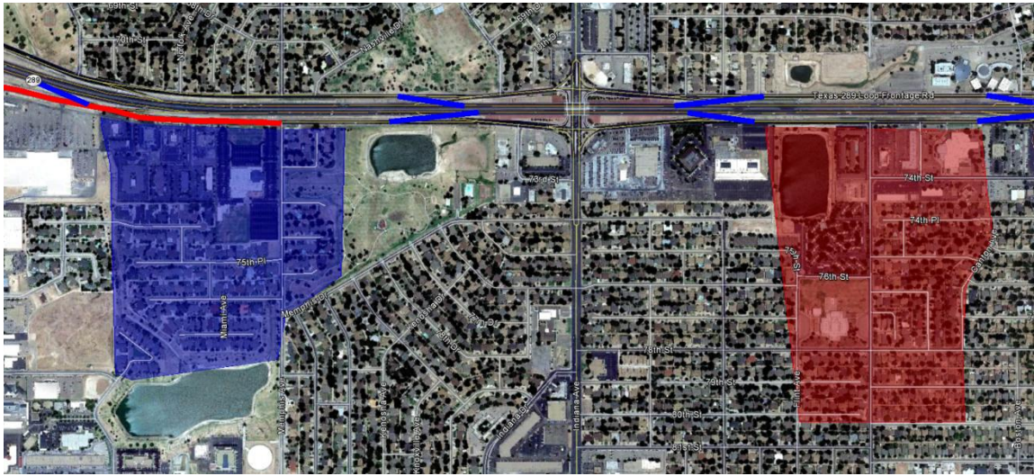
Figure 3-6: Traffic Re-Distribution of the Eastbound Off-Ramp between Quaker Avenue and Indiana Avenue
