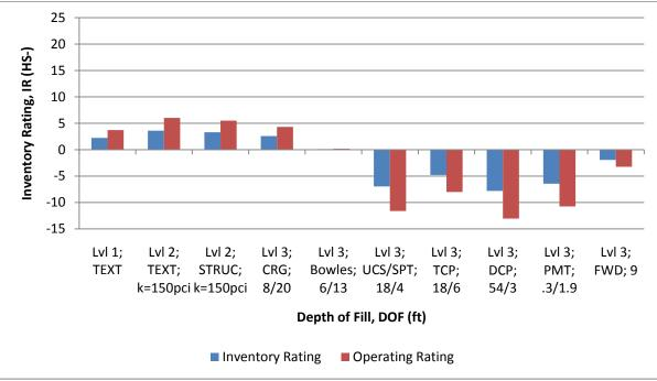
FIGURE 6.31. LOAD RATING FOR TULIA CULVERT: 1.5' OF FILL
