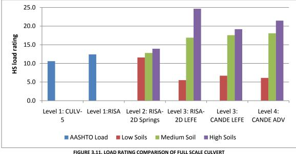
Figure 3.11 shows the comparison of load ratings determined by the different analytical models. For purposes of this analysis, it should be noted that the RISA and CANDE models produce similar rating trends. Results from CANDE using the full array of its concrete models are lower than results from RISA because of CANDE's nonlinear analysis approach.
