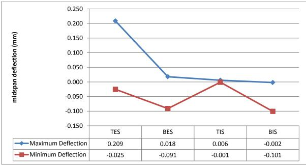
FIGURE 6.36. MEASURED DEFLECTIONS IN MILLIMETERS FOR THE TULIA CULVERT: 1.5' OF FILL
