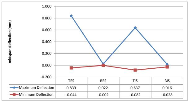
FIGURE 6.14. MEASURED DEFLECTIONS IN MILLIMETERS FOR THE SHALLOWATER CULVERT: 2' OF FILL
