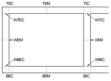
FIGURE 4.7. MOMENT CRITICAL SECTIONS FOR CULVERTS WITHOUT HAUNCHES.
