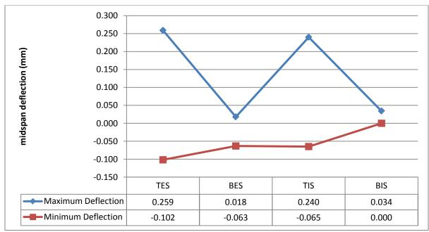
FIGURE 6.28. MEASURED DEFLECTIONS IN MILLIMETERS FOR THE PLAINVIEW CULVERT: 3.5' OF FILL
