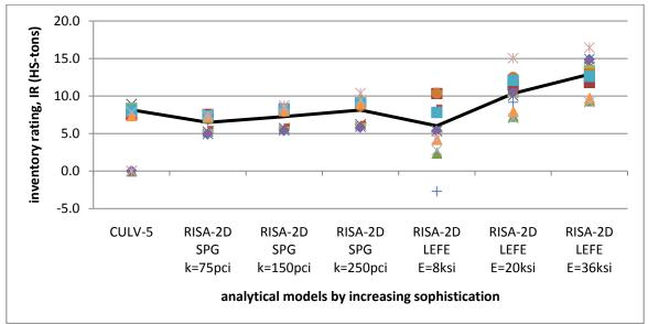
Figure 4.11 and Figure 4.12 show the inventory ratings for medium fill culverts. This subset supports the first hypothesis; RISA-2D with springs produces noticeably higher load ratings than CULV-5. Again the second and third hypotheses are only partial supported. For low soil stiffness the RISA-2D with LEFE produces lower ratings than the CULV-5 and RISA-2D with spring models. However, if the soil is stiff enough, the second and third hypotheses are supported.
