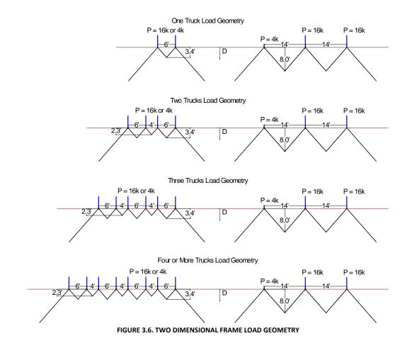
The live load pressures were developed from the load geometries. The worst case scenario was determined for each range by plotting the load factor as a function of trucks and depth. This plot is shown in Figure 3.7 This resulted in the step function outlined in the *Culvert Rating Guide*.
