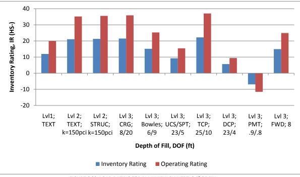
FIGURE 6.23. LOAD RATING FOR PLAINVIEW CULVERT: 3.5' OF FILL
