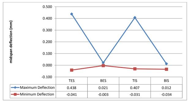
FIGURE 6.20. MEASURED DEFLECTIONS IN MILLIMETERS FOR THE SHALLOWATER CULVERT: 4' OF FILL
