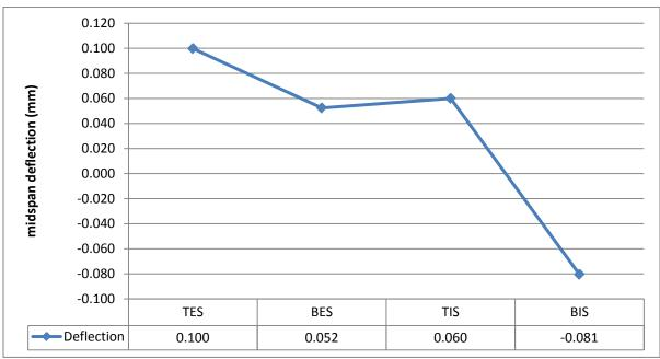
FIGURE 6.39. MEASURED DEFLECTIONS IN MILLIMETERS FOR THE SHALLOWATER CULVERT FROM 2' TO 4' OF FILL
