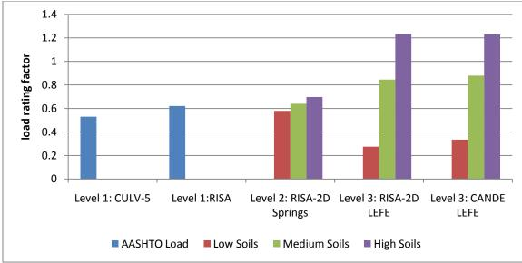
FIGURE 3.12. MOMENT RATING OF FULL SCALE CULVERT
