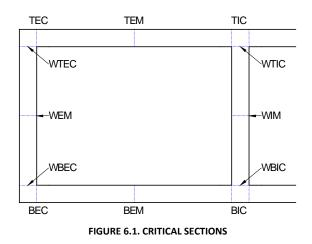
The typical instrumentation plan consisted of placing strain gages at all interior critical sections for both corners and walls. Exterior critical sections were not readily accessible because the culvert is buried; however, critical sections along the top slab could typically be instrumented. In addition to the strain gages, the instrumentation plan included deflection measurements at midspans of the top and bottom slabs.
