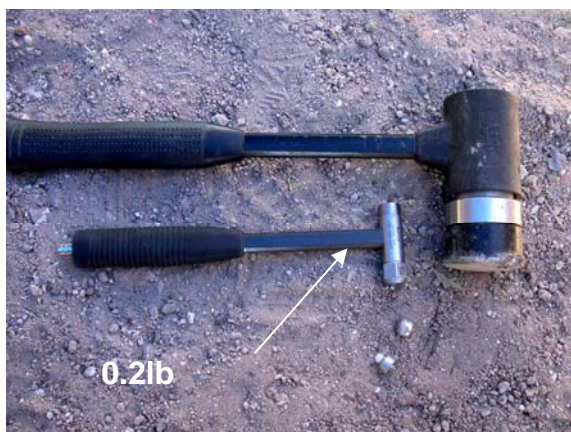
Figure 2 Instrumented Hammer with Interchangeable Metal/Plastic Tips
