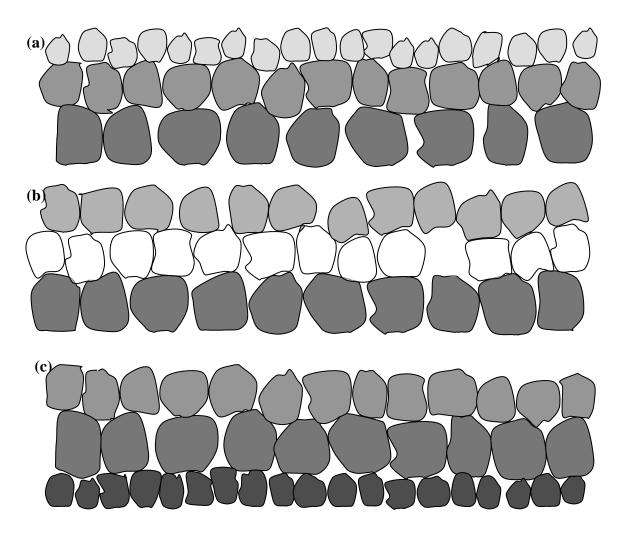
Figure 3.6 Aggregate Grade Combinations Used in 3-CST (a) Grade 5 on Grade 4 on Grade 3 (b) Grade 4 on Grade 4 on Grade 3 (c) Grade 4 on Grade 5.
