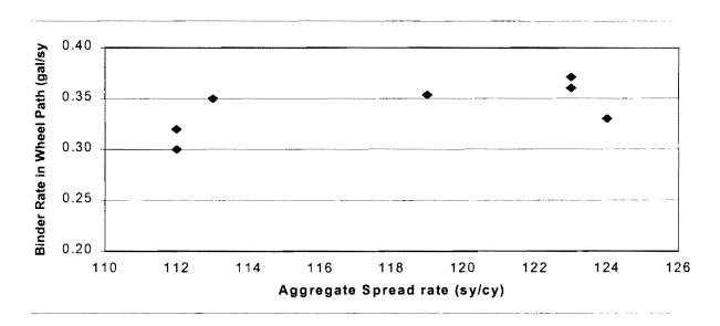
Figure D.5 Binder Rate in Wheel Path vs. Aggregate Rate for AC15-5TR
