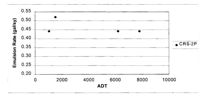
Figure D.4 Emulsion Rate in Wheel Path vs. ADT (Grade 3)
