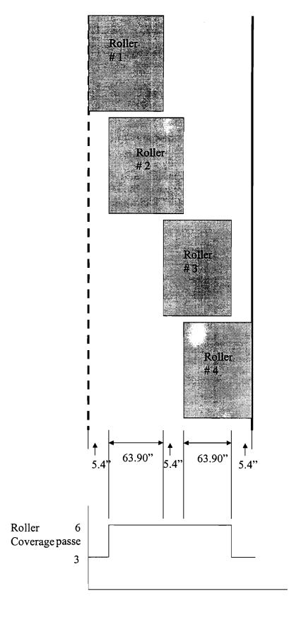
Figure 5.3. Diagonal Pattern and Coverage with Four Medium Rollers
