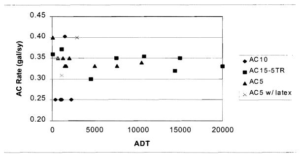
Figure D.1 AC Rate in Wheel Path vs. ADT (Grade 4)
