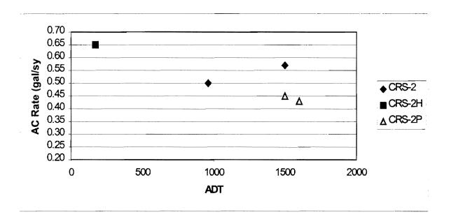
Figure D.2 Emulsion Rate in Wheel Path vs. ADT (Grade 4)
