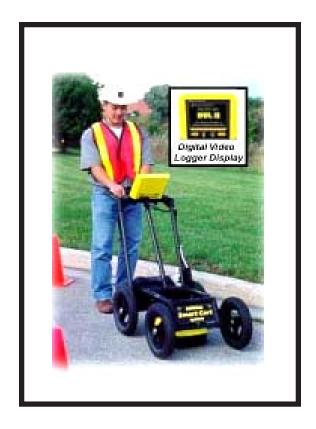
**Figure 3** Nogging Smart Cart from Sensors and Software Inc., in operating mode.
