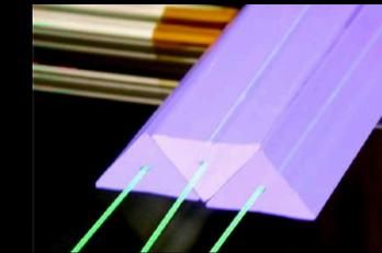
Fig 5. Triangular scintillators
