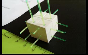
Fig 6. WLS scintillators
